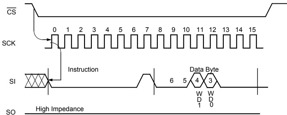
Figure 8. Read Nonvolatile Status (Option 1) (Used to determine end of Watchdog Timer store operation)
