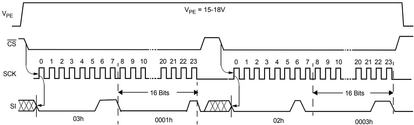
Figure 4.  $V_{TRIP}$  Programming Sequence
