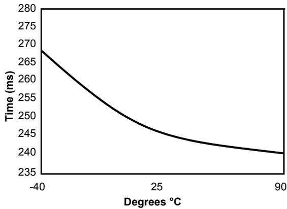
t<sub>WDO</sub> vs. Voltage/Temperature (WD1, 0 0 = 0, 1)
