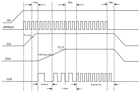
**Figure 4—Startup Sequence Using External Sync Clock Signal**
