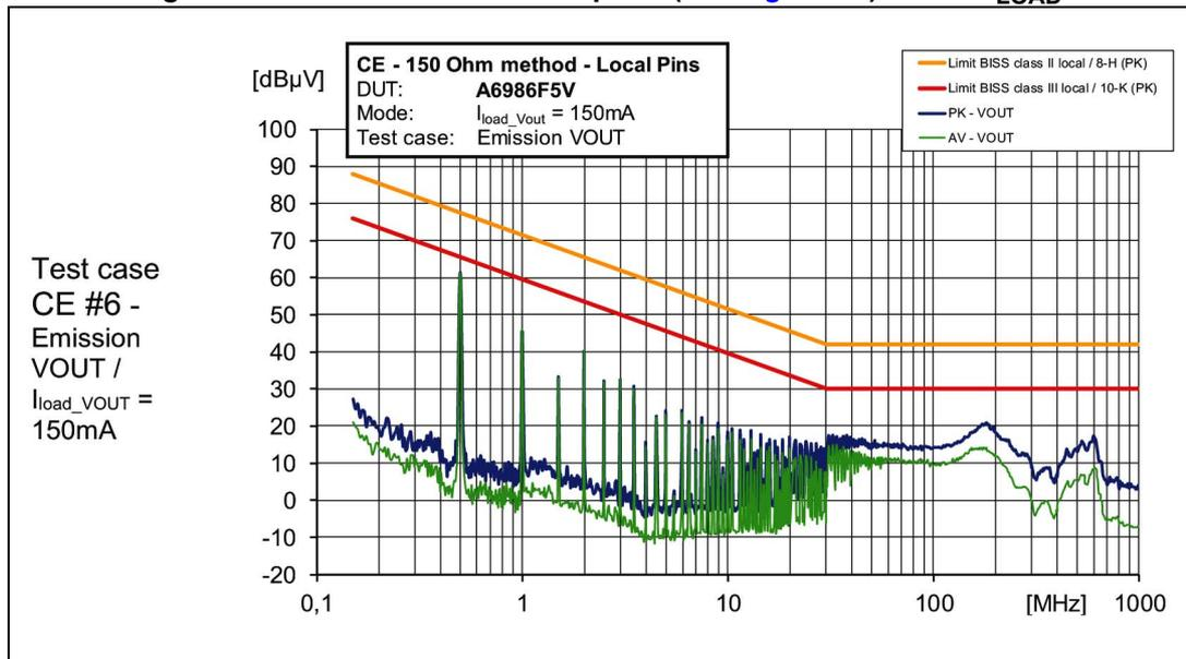
Figure 70. CE 150R at RST test point (see Figure 65) at 80% I<sub>LOAD</sub>
