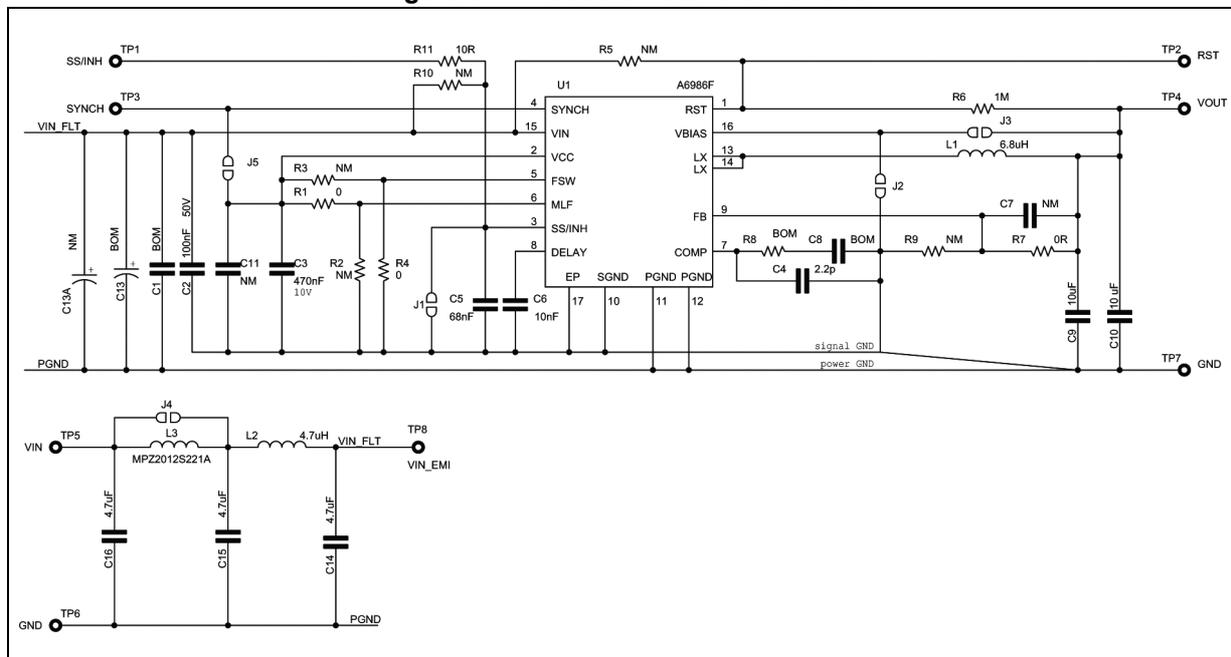
The additional input filter (C16, L3, C15, L2, C14) limits the conducted emission on the power supply (refer to [Section 10 on page 69](#)).
