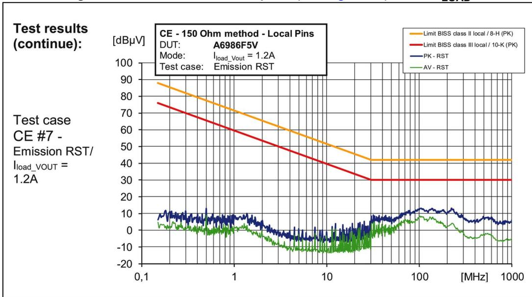
Figure 71. CE 150R at RST test point (see Figure 65) at 10% I<sub>LOAD</sub>
