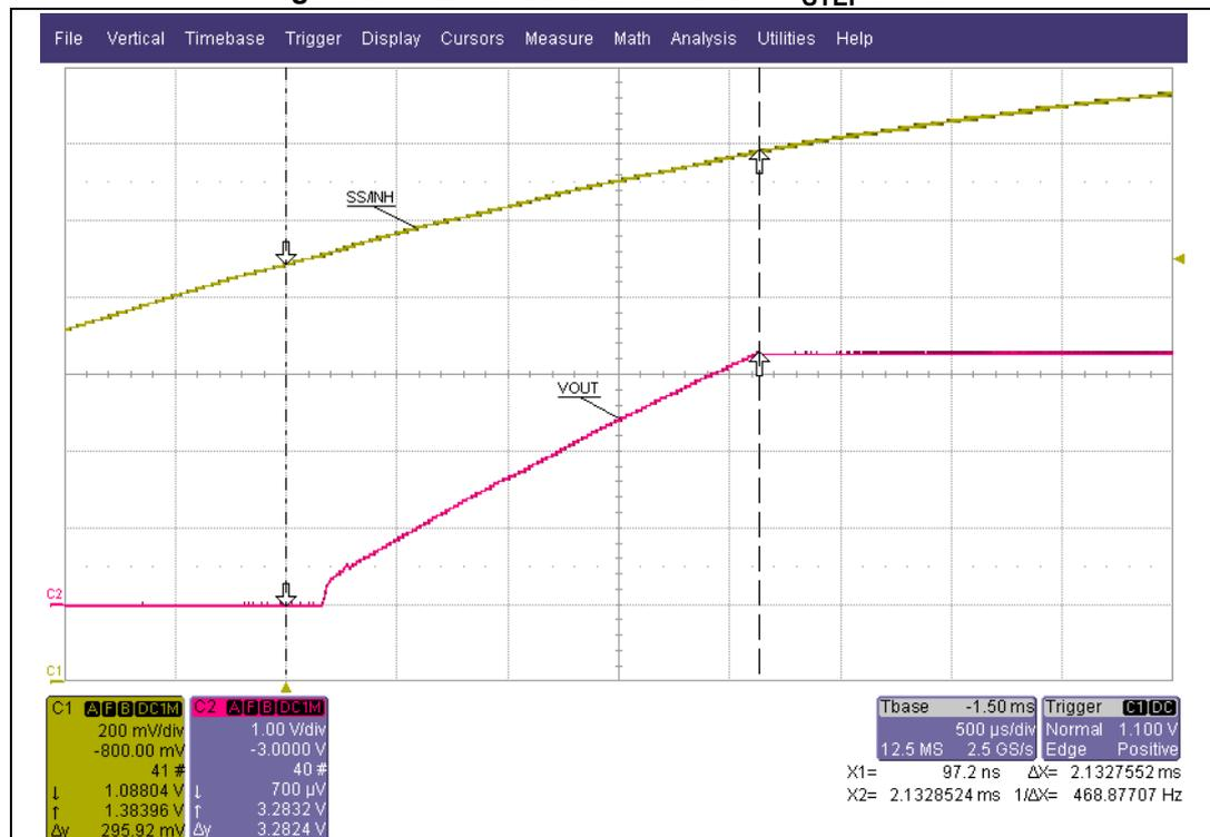
The circuit in *Figure 7* introduces a time delay between  $V_{STEP}$  and the switching activity that can be calculated as:
