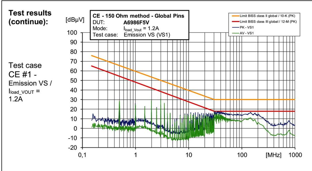
Figure 67. CE 150R at VS1 test point (see [Figure 65](#)) at 10% I<sub>LOAD</sub>
