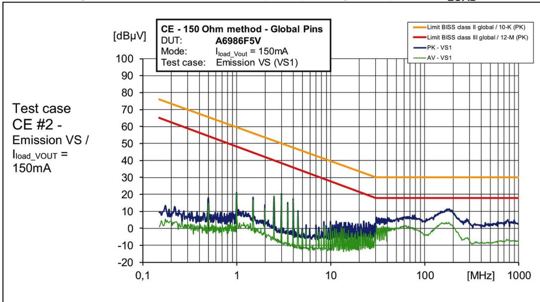
Figure 68. CE 150R at VOUT test point (see Figure 65) at 80% I<sub>LOAD</sub>
