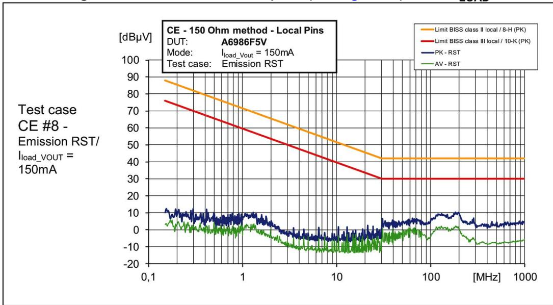
Figure 72. CE 150R at SS/INH test point (see Figure 65 on page 70) at 80% I<sub>LOAD</sub>
