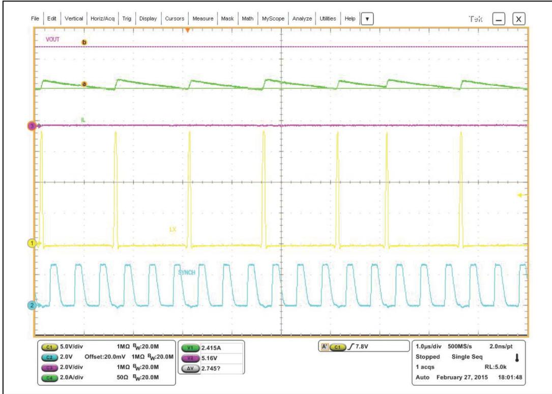
Figure 30 shows the switching frequency reduction during the valley current sense operation in case of extremely low duty cycle ( $V_{IN} = 38\text{ V}$ ,  $f_{SW} = 500\text{ kHz}$  short-circuit condition).
