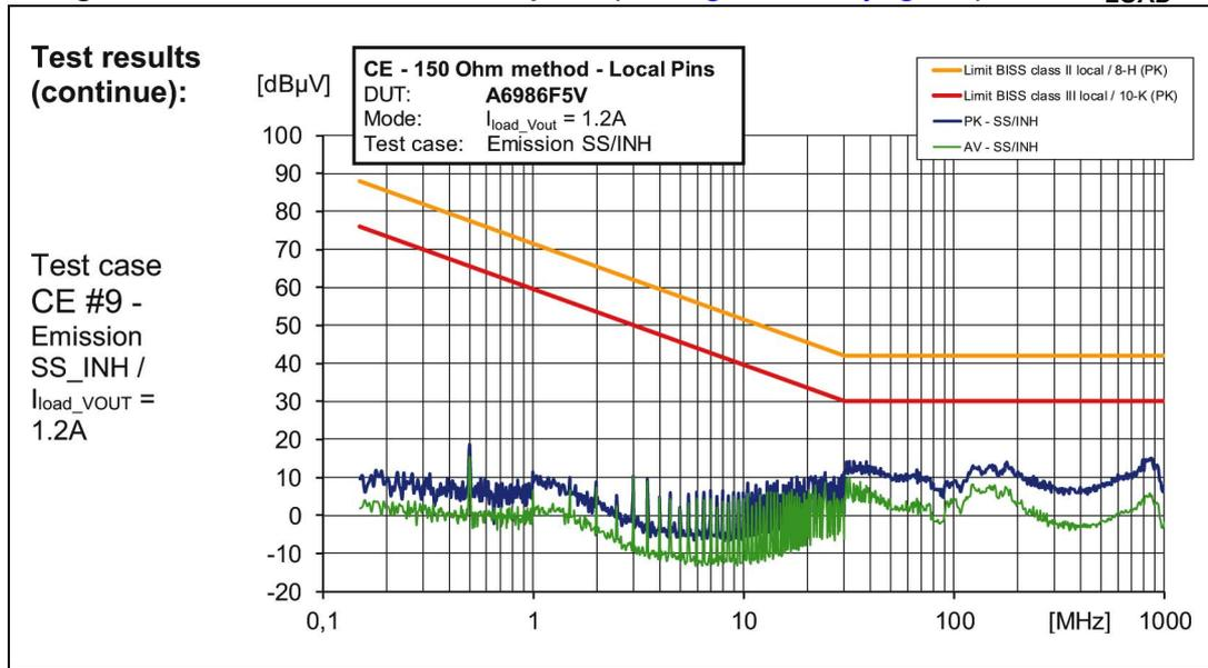
Figure 73. CE 150R at SS/INH test point (see Figure 65) at 10% I<sub>LOAD</sub>
