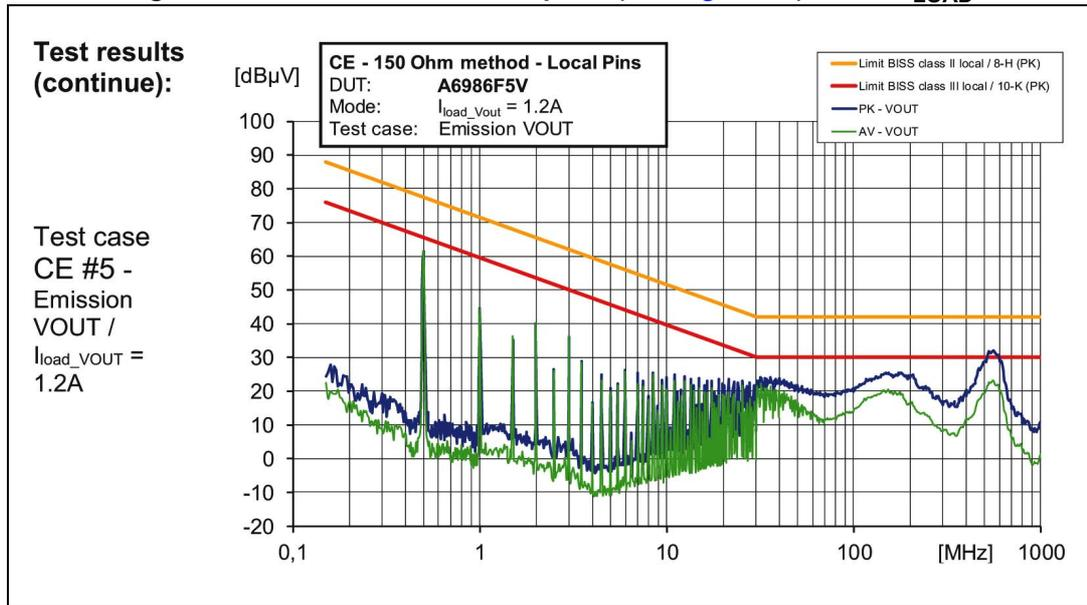
Figure 69. CE 150R at VOUT test point (see Figure 65) at 10% I<sub>LOAD</sub>
