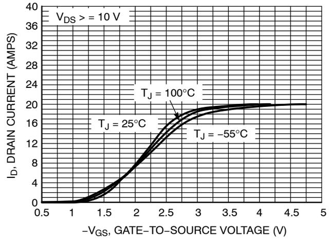
**Figure 2. Transfer Characteristics**
