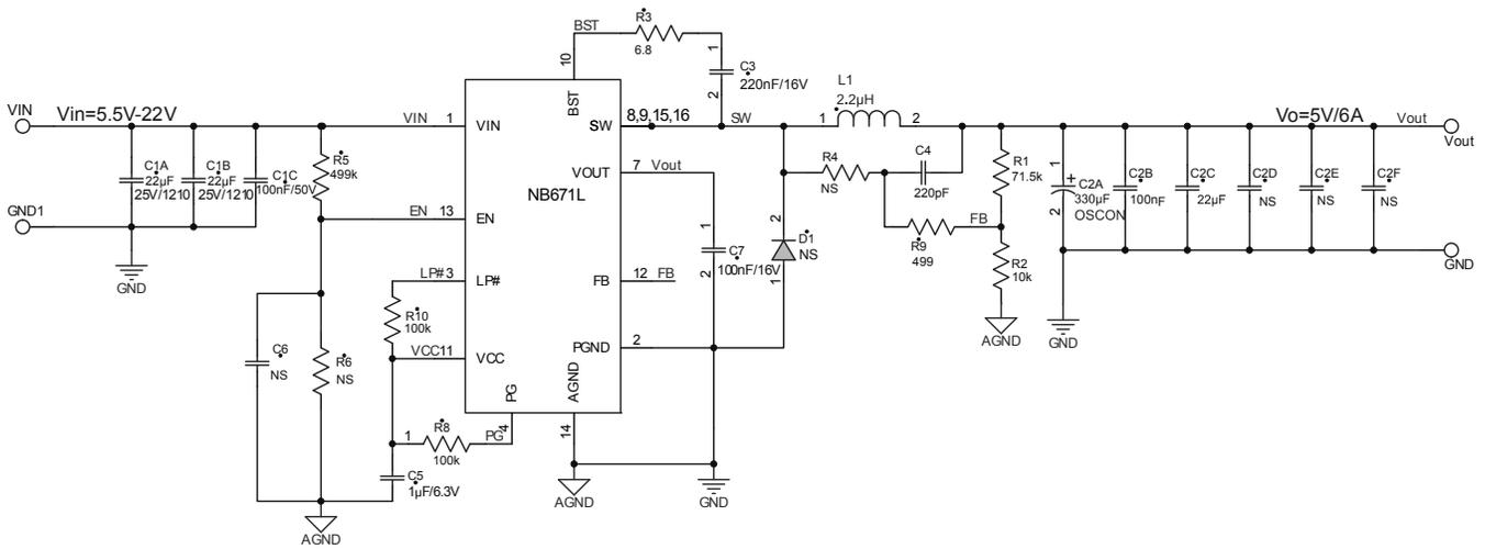
**Figure 14 — Typical Application Circuit For NB671L**
