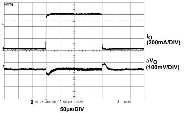
**FIGURE 17. PWM LOAD TRANSIENT RESPONSE (30mA TO 600mA)**
