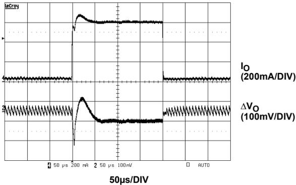
**FIGURE 16. LOAD TRANSIENT RESPONSE (22mA TO 600mA)**
