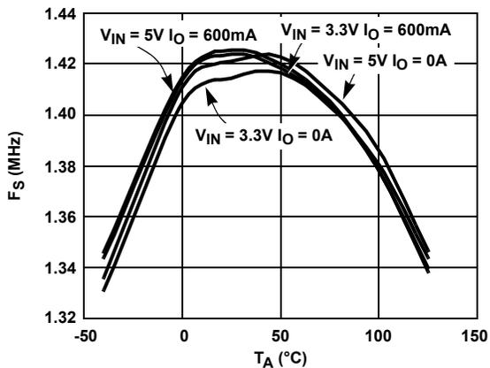
FIGURE 5.  $F_S$  vs JUNCTION TEMPERATURE (PWM MODE)
