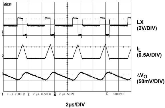
**FIGURE 12. PFM STEADY-STATE OPERATION WAVEFORM ( $I_O = 100mA$ )**
