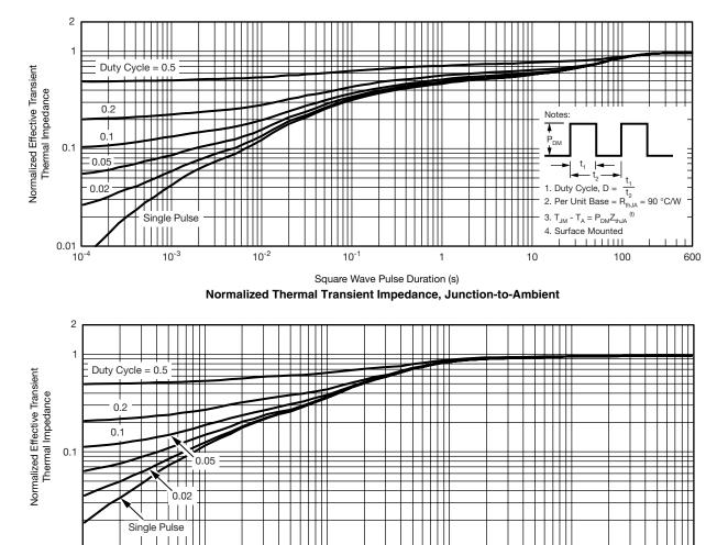
Square Wave Pulse Duration (s) Normalized Thermal Transient Impedance, Junction-to-Foot
