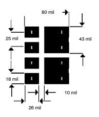
FIGURE 2. Footprint With Copper Spreading
