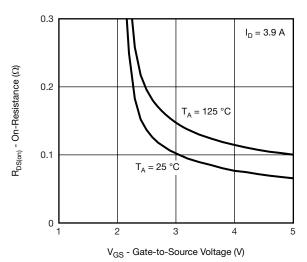
On-Resistance vs. Gate-to-Source Voltage
