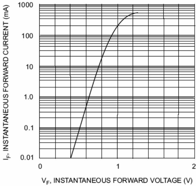
Fig. 1 Forward Characteristics
