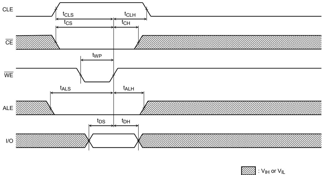
Address Input Cycle Timing Diagram
