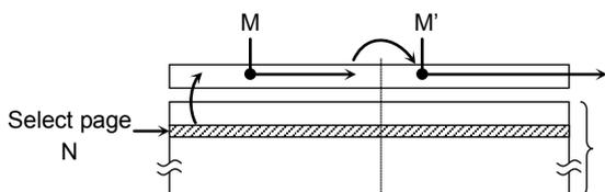
During the serial data output from the register, the column address can be changed by inputting a new column address using the 05h and E0h commands. The data is read out in serial starting at the new column address. Random Column Address Change operation can be done multiple times within the same page.
