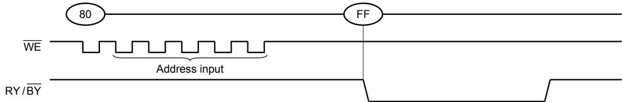
If a command other than “85h”, “10h”, “11h” or “FFh” is input, the Program operation is not performed and the device operation is set to the mode which the input command specifies.
