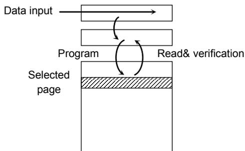
The data is transferred (programmed) from the Data Cache via the Page Buffer to the selected page on the rising edge of  $\overline{WE}$  following input of the "10h" command. After programming, the programmed data is transferred back to the Page Buffer to be automatically verified by the device. If the programming does not succeed, the Program/Verify operation is repeated by the device until success is achieved or until the maximum loop number set in the device is reached.
