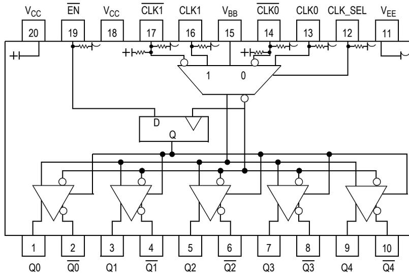
Warning: All  $V_{CC}$  and  $V_{EE}$  pins must be externally connected to Power Supply to guarantee proper operation.
