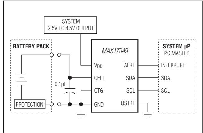
Figure 15. MAX17049 Application Circuit (2S Cell Pack)
