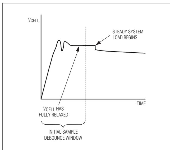
Figure 6. Insertion Waveform Not Requiring Quick-Start Command
