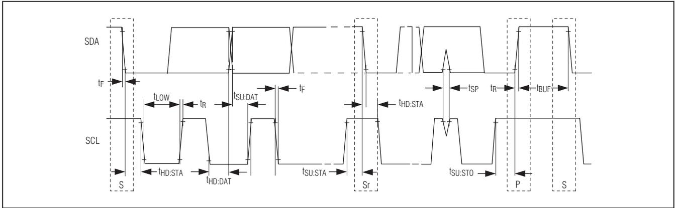
Figure 1. I<sup>2</sup>C Bus Timing Diagram
