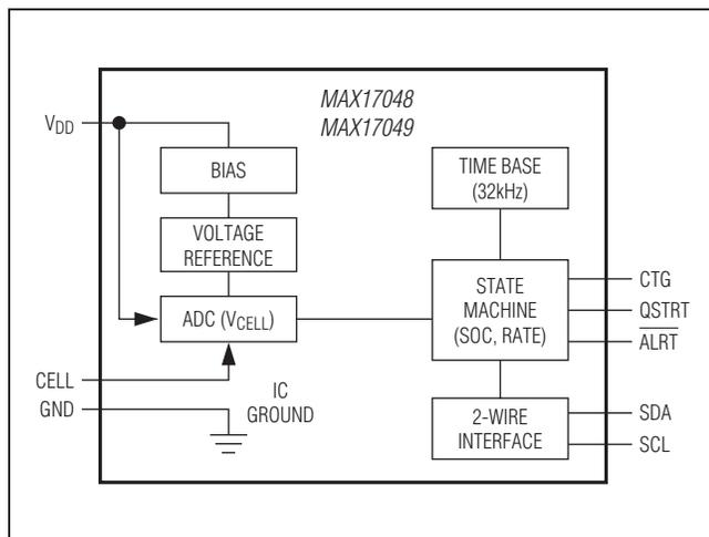
Figure 2. Block Diagram
