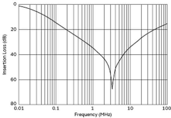
Differential Mode Insertion Loss (Typ.)
