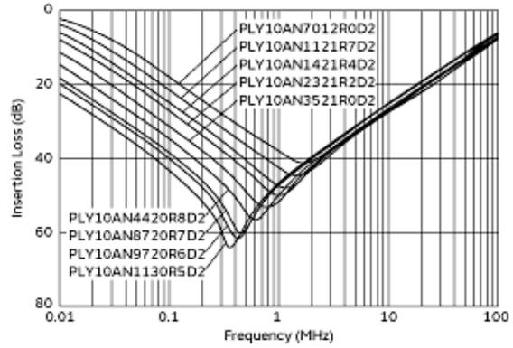
Common Mode Insertion Loss-Frequency Characteristics
