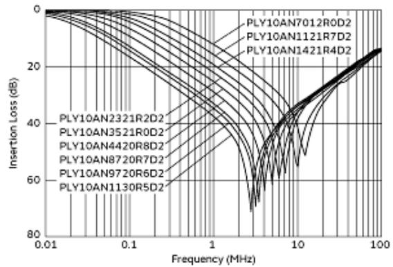
Differential Mode Insertion Loss-Frequency Characteristics
