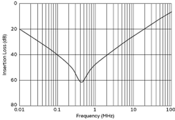
Common Mode Insertion Loss (Typ.)
