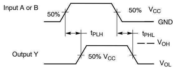
**Figure 3. Switching Waveforms**
