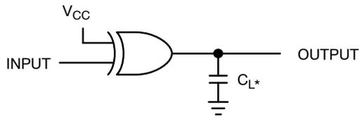
\*Includes all probe and jig capacitance.
