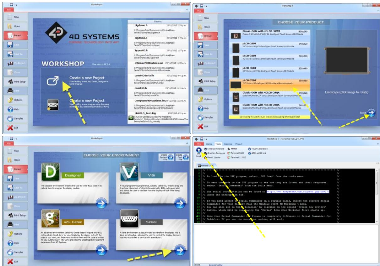
In the 'Tools' menu of the Serial Environment, is a button called 'SPE Load'. SPE stands for "Serial Platform Environment". If your display module is connected to the PC via the 4D Systems Programming Cable, clicking this button will load a special 4DGL application onto your module. This application is known as the SPE Application, and will enable your chosen module to run as a Serial Slave.
