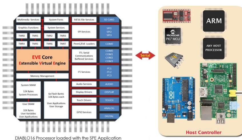
**Serial Data Format: 8 Bits, No Parity, 1 Stop Bit. Serial data is true and not inverted.**
