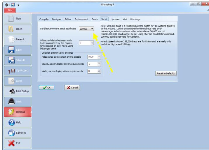
The initial Baud rate and 'slowdown' settings for slow systems can be set under 'options', 'serial' before loading SPE.
