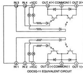
DC INDUCTIVE LOADS MUST BE DIODE SUPPRESSED TO PREVENT DAMAGE TO THE I/O MODULE.
