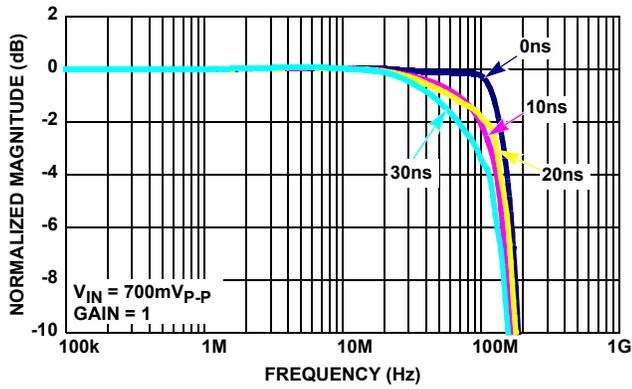
FIGURE 9. ISL59923 FREQUENCY RESPONSE (GAIN = 1)
