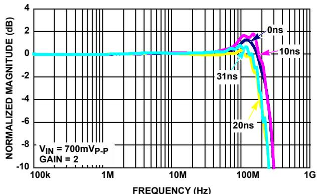
FIGURE 8. ISL59922 FREQUENCY RESPONSE (GAIN = 2)
