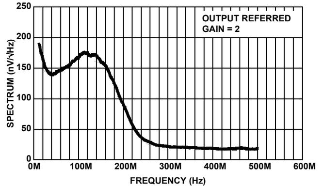
FIGURE 12. ISL59920 NOISE SPECTRUM (10k TO 500MHz)
