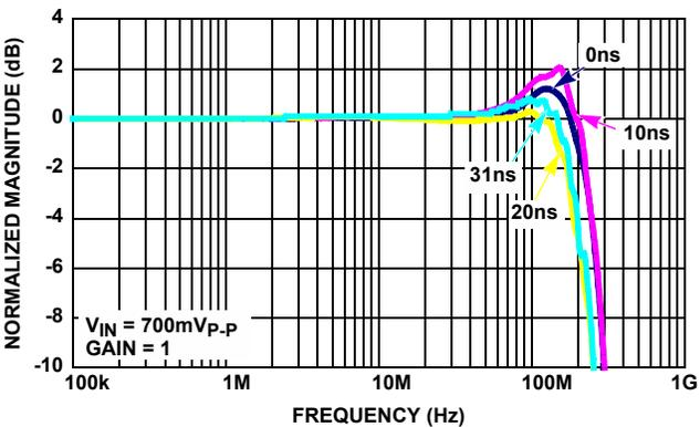
FIGURE 7. ISL59922 FREQUENCY RESPONSE (GAIN = 1)
