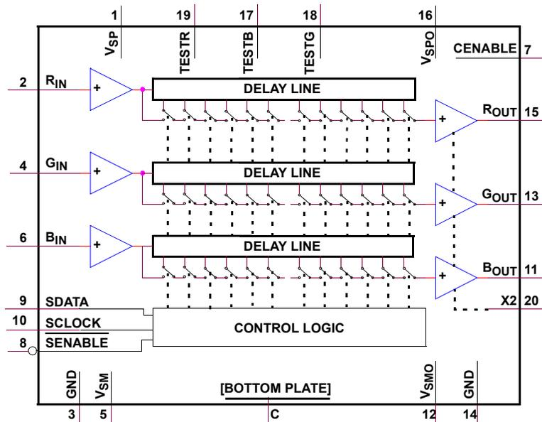
FIGURE 1. ISL59920, ISL59921, ISL59922, ISL59923 BLOCK DIAGRAM
