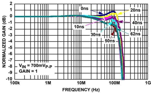
FIGURE 3. ISL59920 FREQUENCY RESPONSE (GAIN = 1)
