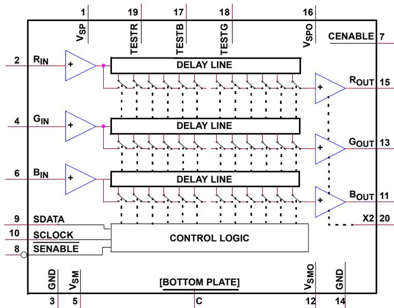
FIGURE 34. ISL59920, ISL59921, ISL59922, ISL59923 BLOCK DIAGRAM
