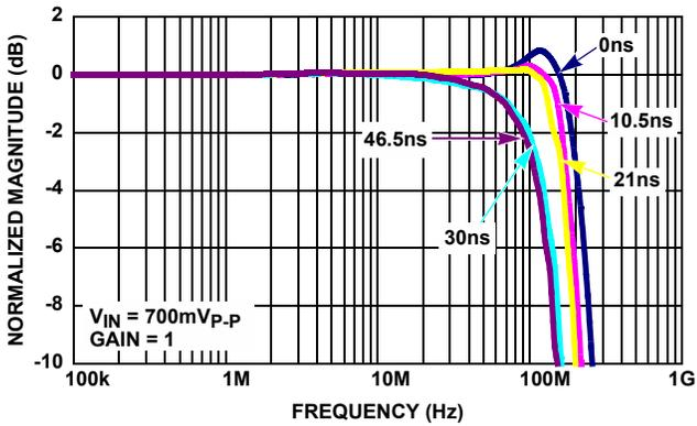
FIGURE 5. ISL59921 FREQUENCY RESPONSE (GAIN = 1)
