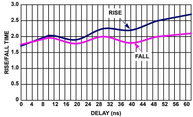
FIGURE 16. ISL59920 RISE/FALL TIME vs DELAY TIME (GAIN = 2)
