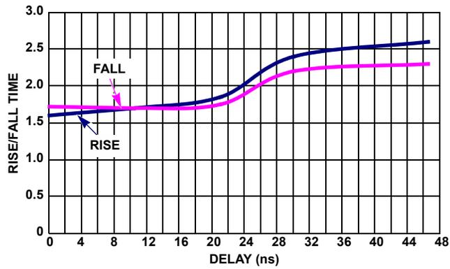
FIGURE 17. ISL59921 RISE/FALL TIME vs DELAY TIME (GAIN = 2)
