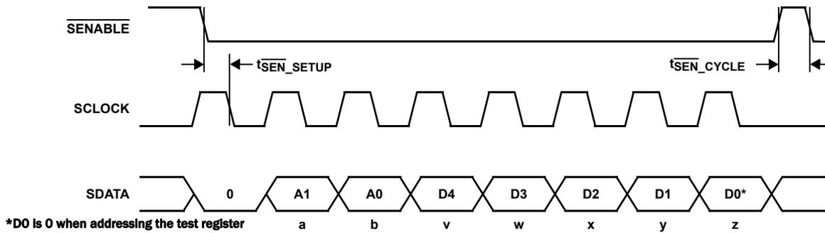
FIGURE 35. SERIAL TIMING
