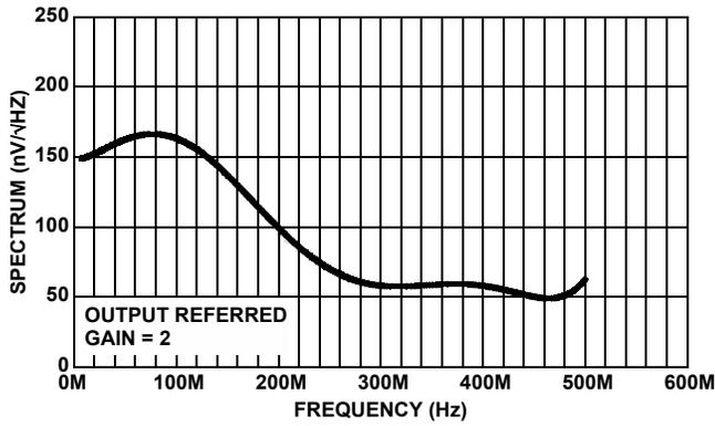
FIGURE 15. ISL59923 NOISE SPECTRUM (10k TO 500MHz)
