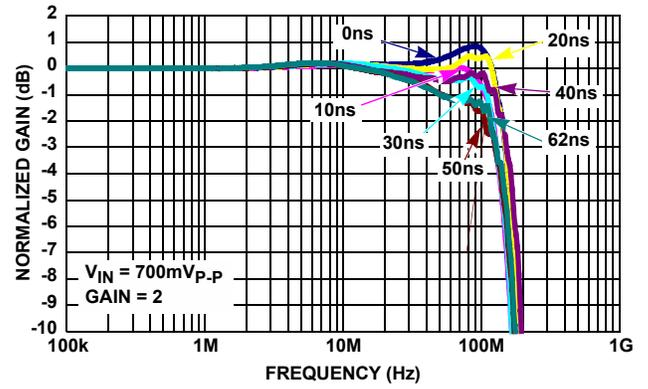
FIGURE 4. ISL59920 FREQUENCY RESPONSE (GAIN = 2)
