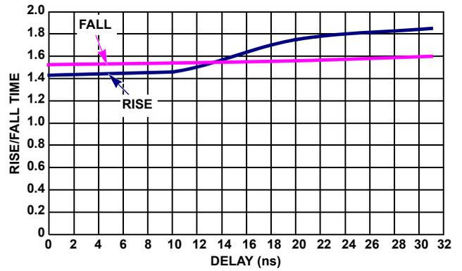
FIGURE 18. ISL59922 RISE/FALL TIME vs DELAY TIME (GAIN = 2)
