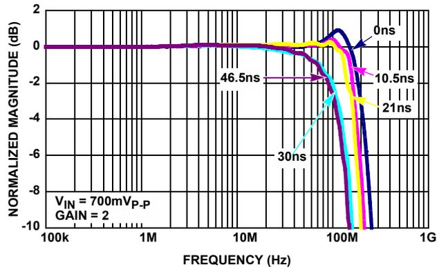
FIGURE 6. ISL59921 FREQUENCY RESPONSE (GAIN = 2)
