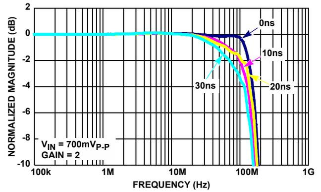
FIGURE 10. ISL59923 FREQUENCY RESPONSE (GAIN = 2)
