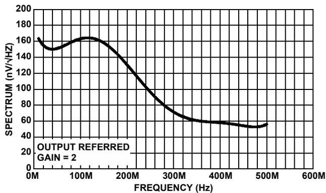
FIGURE 13. ISL59921 NOISE SPECTRUM (10k TO 500MHz)
