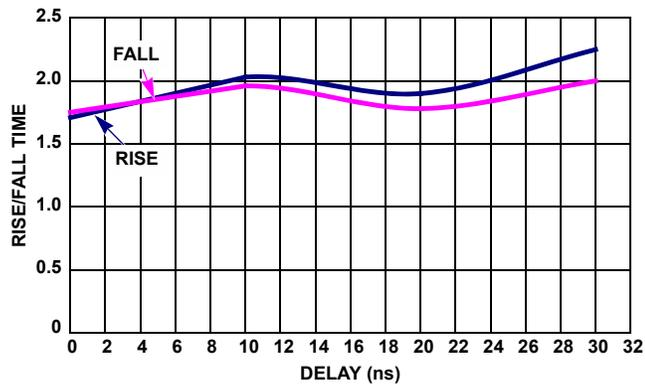
FIGURE 19. ISL59923 RISE/FALL TIME vs DELAY TIME (GAIN = 2)
