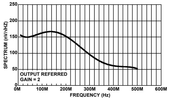
FIGURE 14. ISL59922 NOISE SPECTRUM (10k TO 500MHz)
