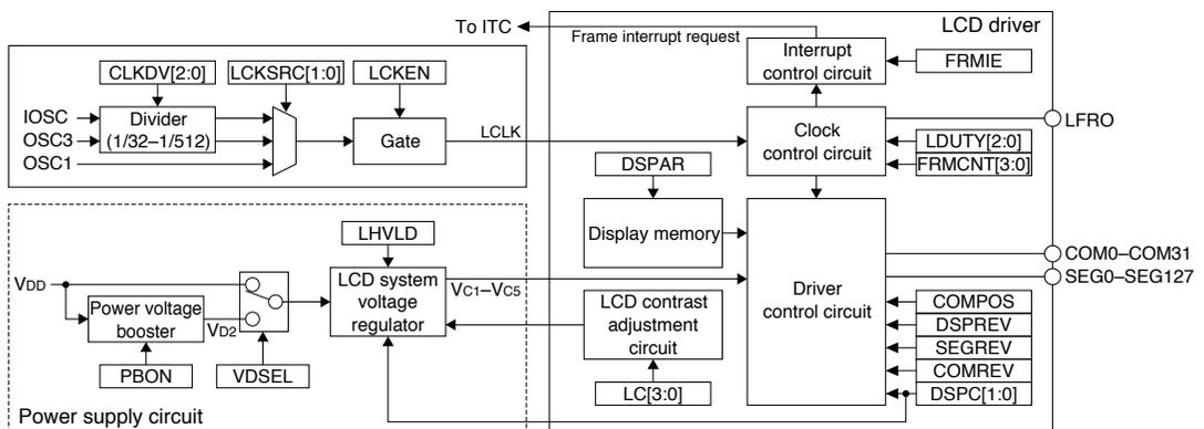
Figure 19.1.1 LCD Driver and Driver Power Supply Configuration
