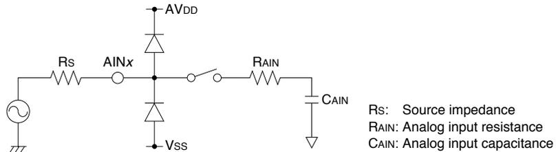
Figure 20.3.5.1 Equivalent Circuit of Analog Input Portion
