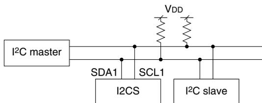
Figure 17.2.1 I<sup>2</sup>C Connection Example
