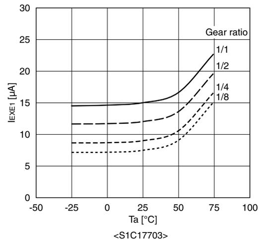
**Current consumption-frequency characteristic during execution with OSC3**
