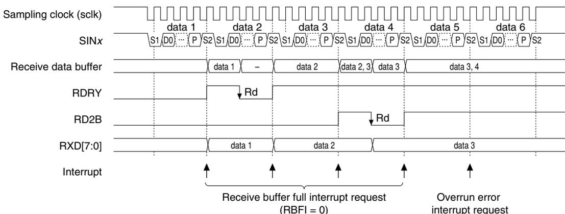
S1: Start bit, S2: Stop bit, P: Parity bit, Rd: Data read from RXD[7:0]
