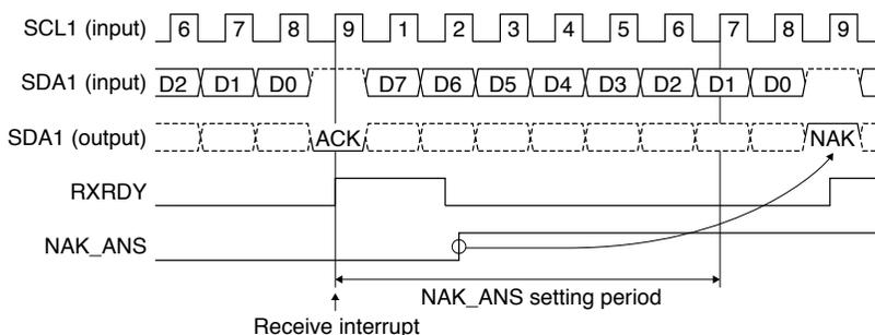
Figure 17.5.3 NAK\_ANS Setting and NAK Response Timing
