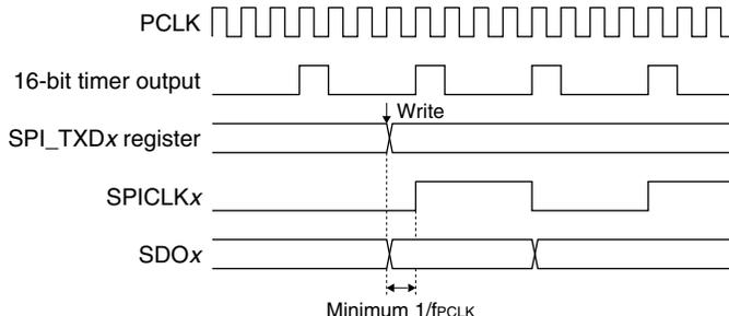
Figure 15.5.1 SDOx and SPICLKx Change Timings when CPHA = 0
