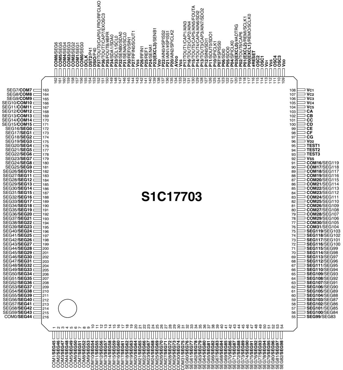
Figure 1.3.2.1 S1C17703 Pin Configuration Diagram (QFP21-216pin)
