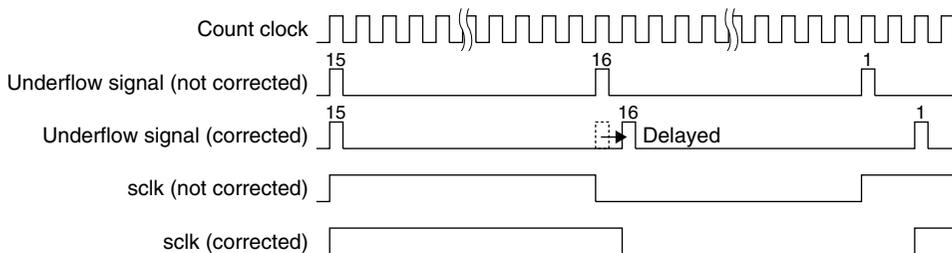
Figure 14.3.3 Delay Cycle Insertion in Fine Mode
