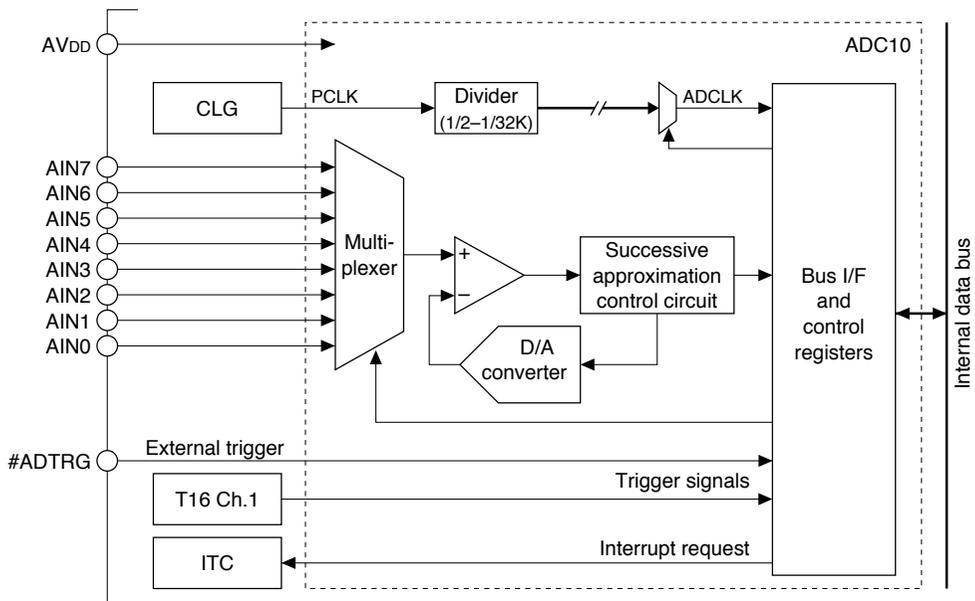
Figure 20.1.1 A/D Converter Configuration
