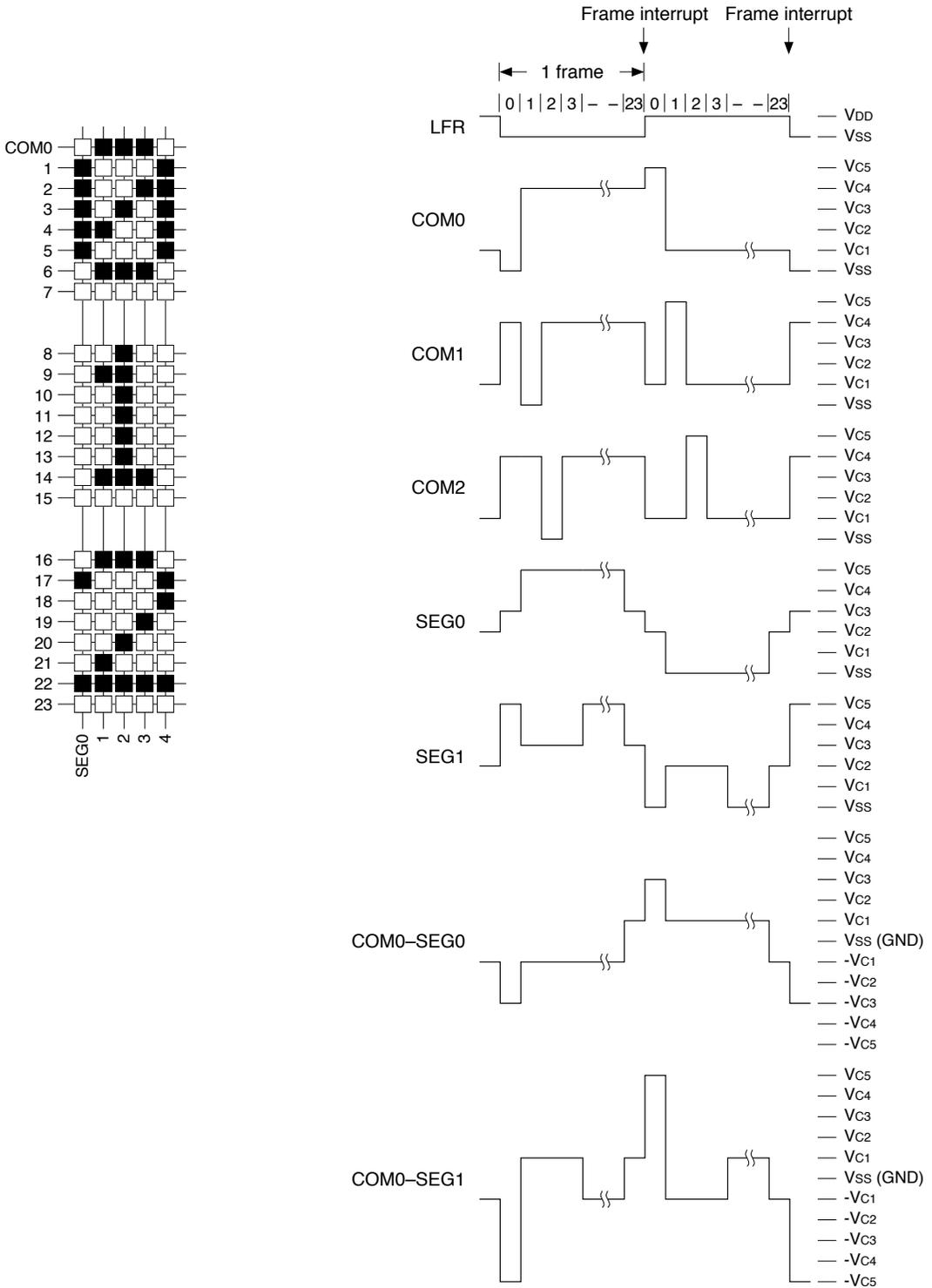
Figure 19.5.2.2 1/24 Duty Drive Waveform
