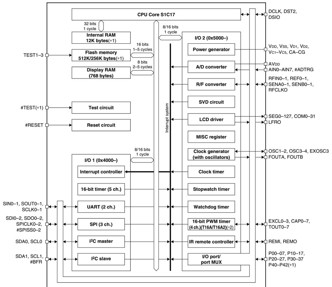
Figure 1.2.1 Block Diagram
