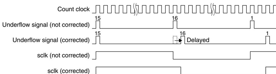
Figure 14.9.1 Delay Cycle Insertion in Fine Mode
