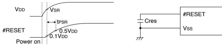
**Note:** Be sure to set the #RESET pin to 0.1 V<sub>DD</sub> or less when performing a power-on reset after the power is turned off.
