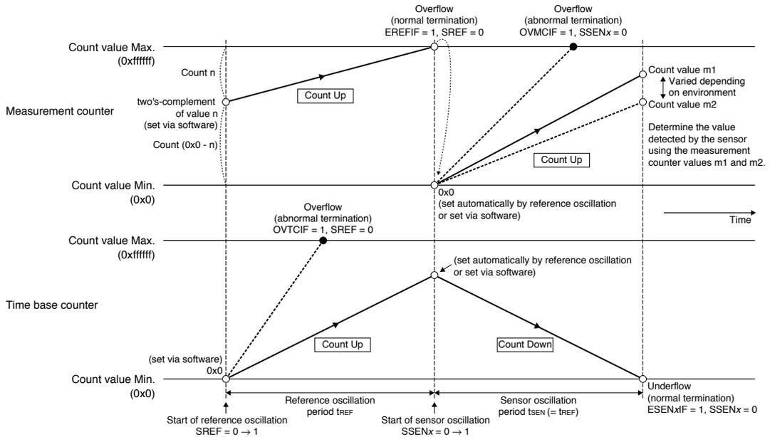
Figure 21.6.2.1 Counter Operations During Reference/Sensor Oscillation
