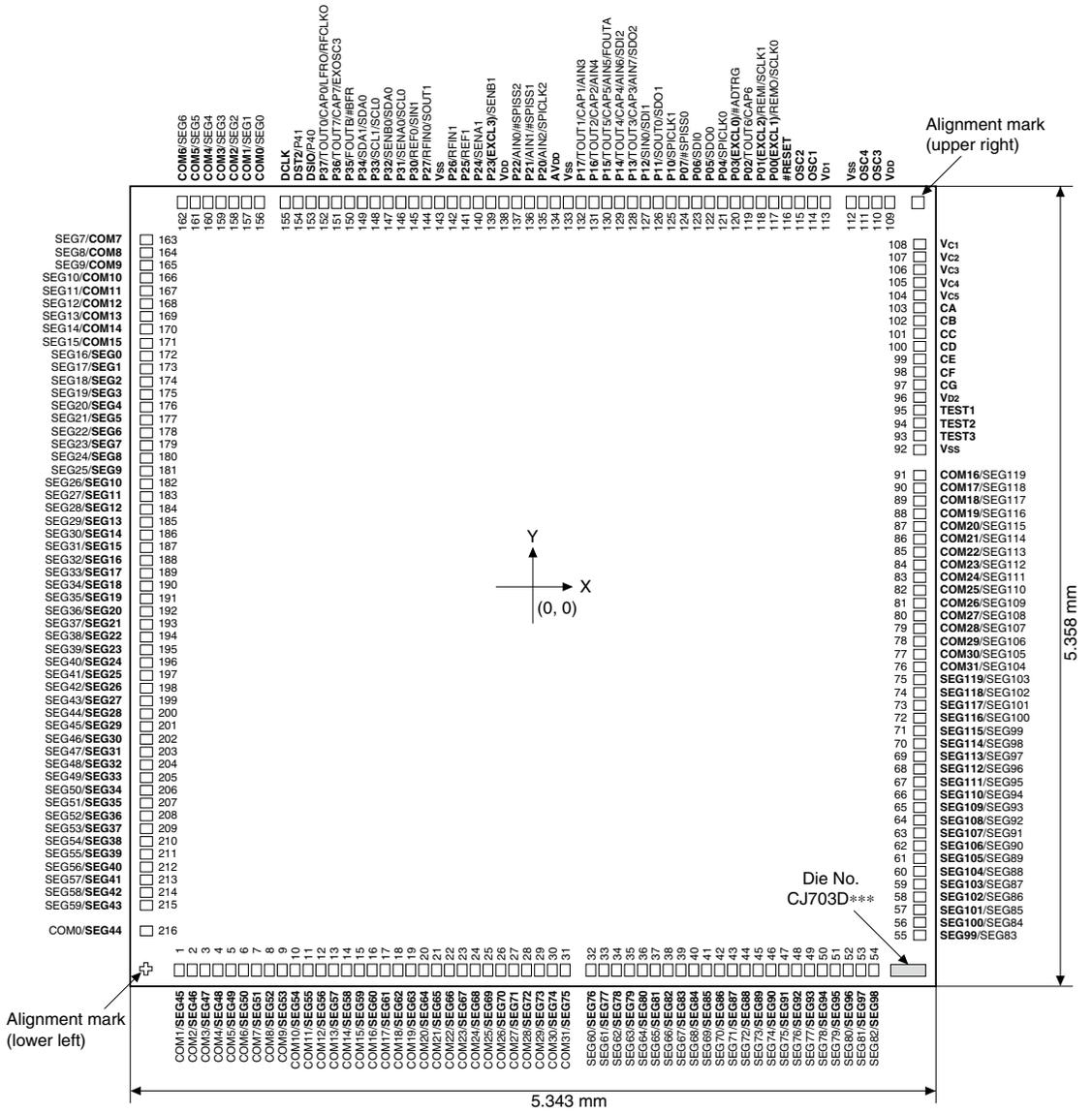
Pad opening No. 1 to 54, 109 to 162: 67.4 × 85 μm
