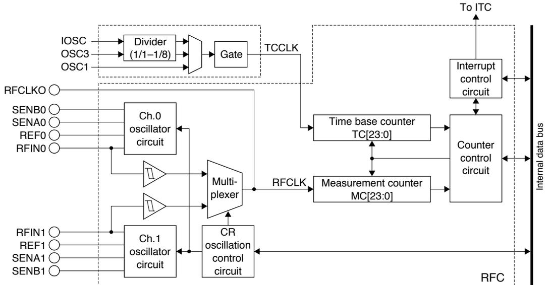
Figure 21.1.1 R/F Converter Configuration
