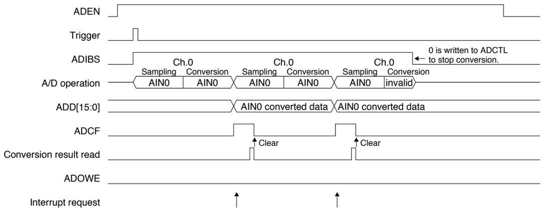
(3) Single channel (AIN0) continuous conversion mode (ADCS = 0, ADCE = 0, ADMS = 1)
