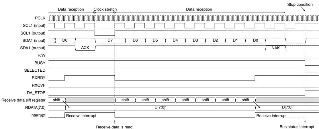
Figure 17.5.8 I2CS Timing Chart 4 (data reception → stop condition)
