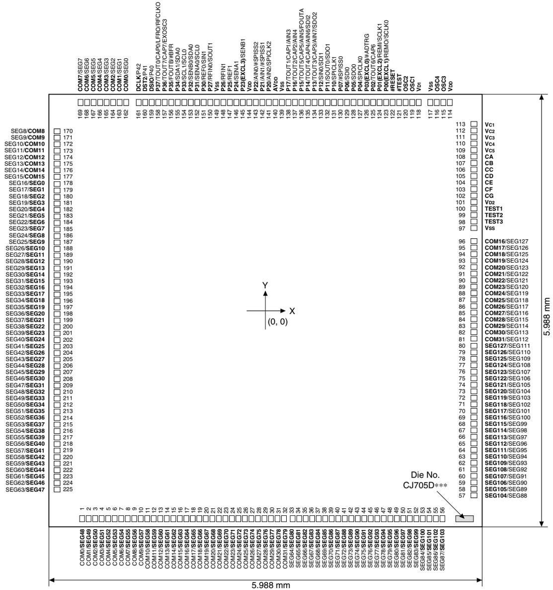
Pad opening No. 1 to 56, 114 to 169: 68 × 85 μm
