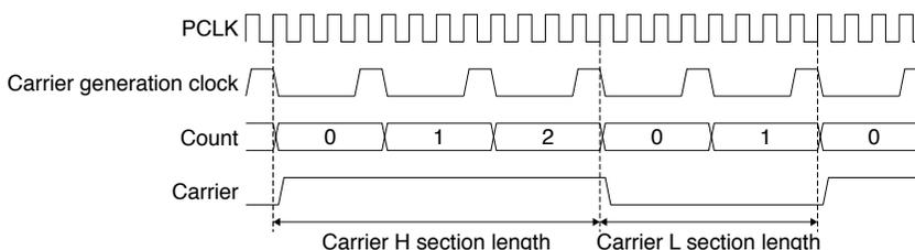
Figure 18.7.1 Carrier Signal Generation
