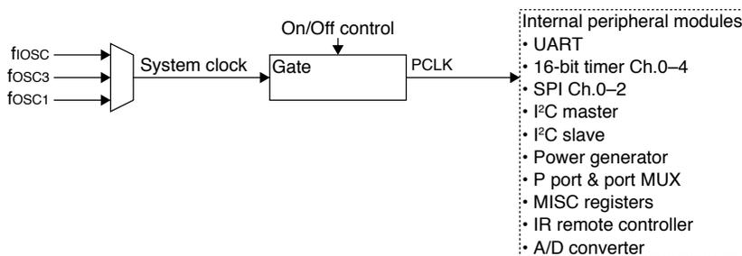
Figure 7.6.1 Peripheral Module Clock Control Circuit
