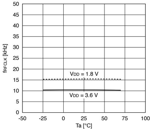
**RFC reference/sensor oscillation frequency-temperature characteristic
