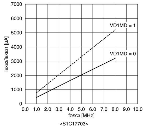
**Current consumption-frequency characteristic during execution with OSC3 + clock gear**
