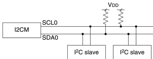
Figure 16.2.1 I<sup>2</sup>C Connection Example
