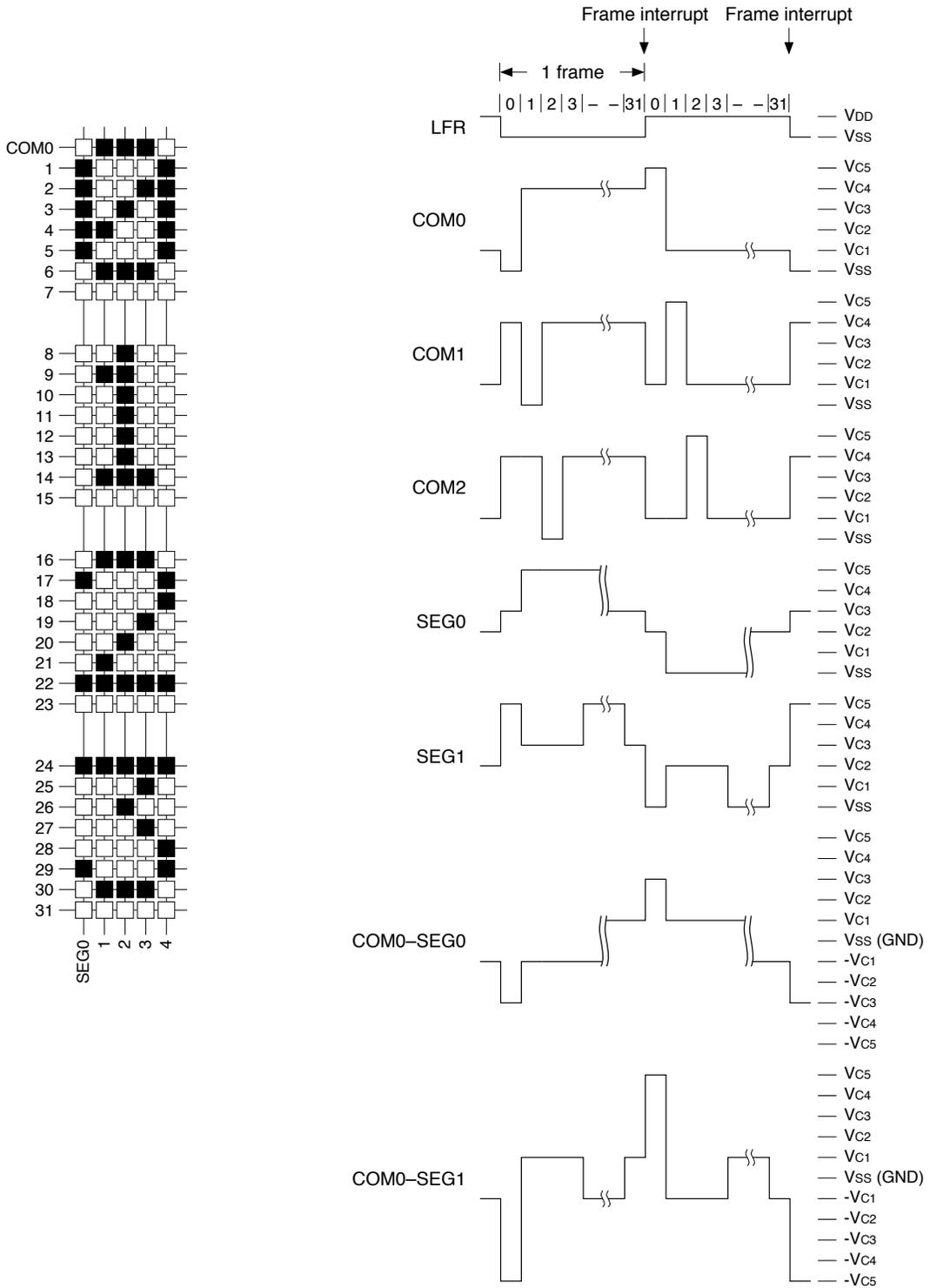
Figure 19.5.2.1 1/32 Duty Drive Waveform
