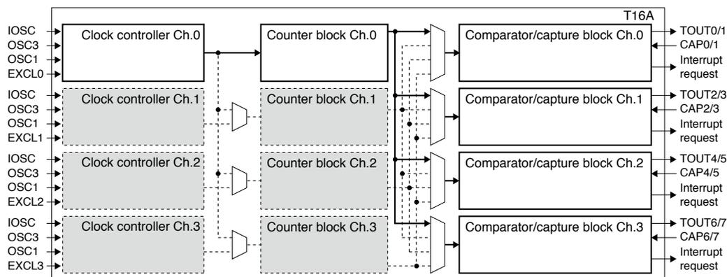
(2) Configuration Example 2 (eight comparator/capture blocks × one channel)
