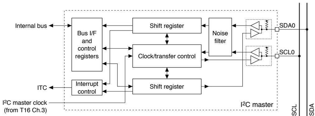
Figure 16.1.1 I2CM Module Configuration
