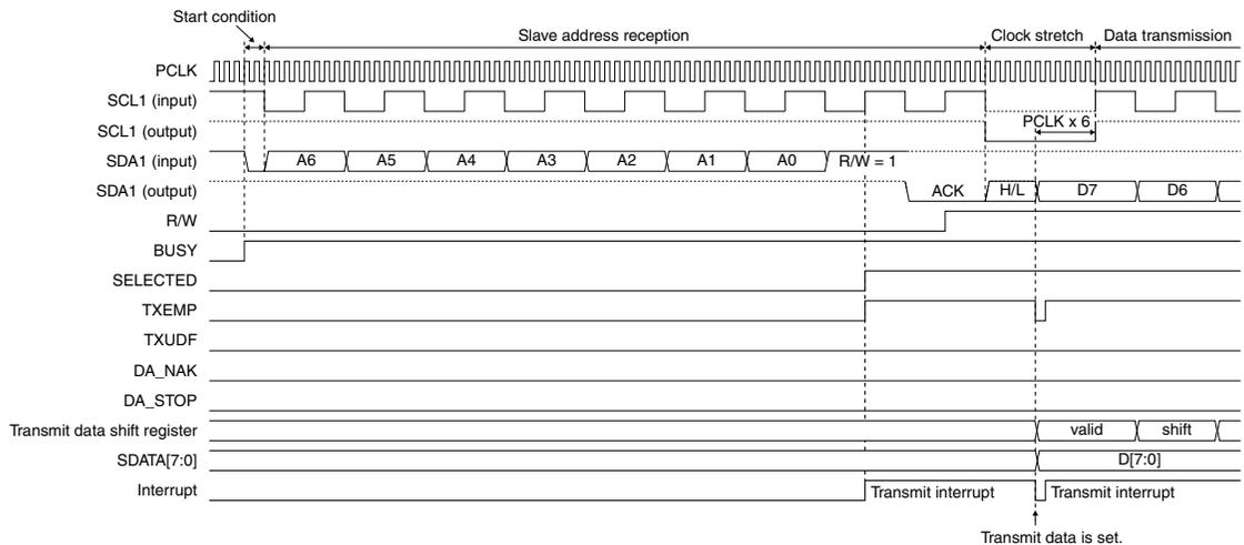
Figure 17.5.5 I<sup>2</sup>C Timing Chart 1 (start condition → data transmission)
