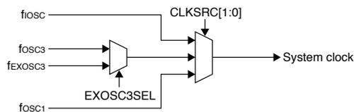
Figure 7.4.1 System Clock Selector
