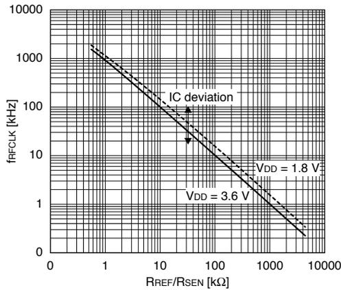
**RFC reference/sensor oscillation frequency-capacitance characteristic
