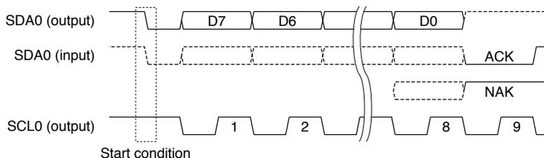
Figure 16.5.3 ACK and NAK
