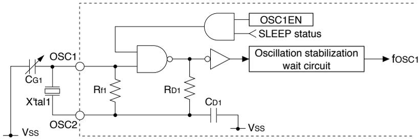
Figure 7.3.3.1 OSC1 Oscillator Circuit
