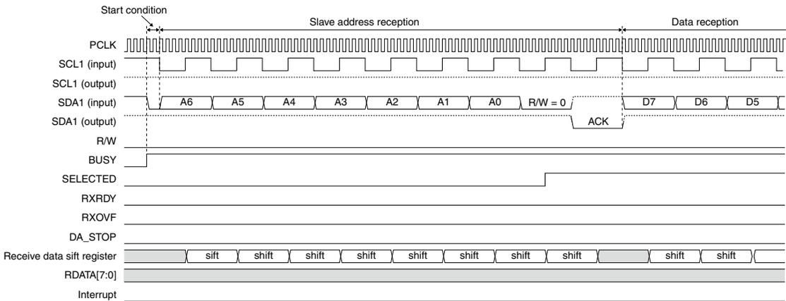
Figure 17.5.7 I2CS Timing Chart 3 (start condition → data reception)
