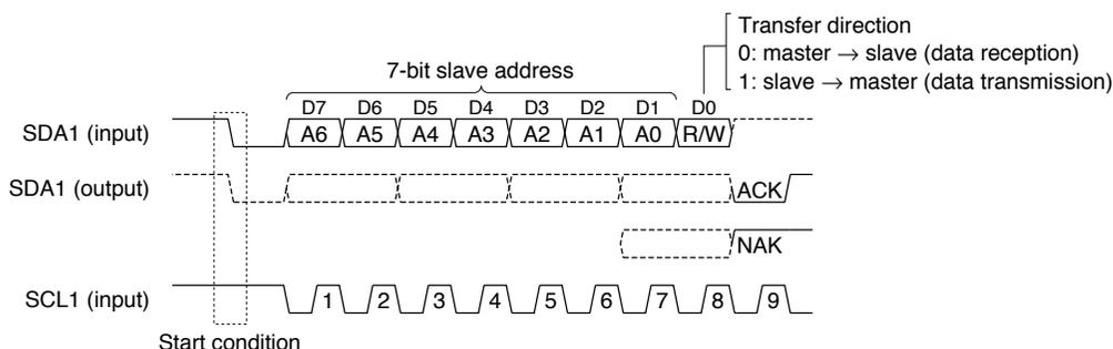
Figure 17.5.1 Receiving Slave Address and Data Direction Bit
