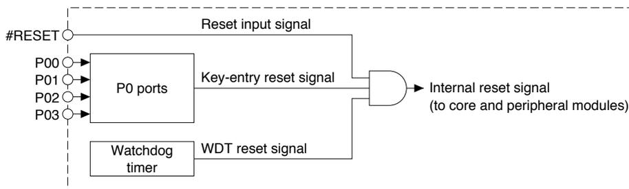
Figure 5.1.1 Configuration of Initial Reset Circuit
