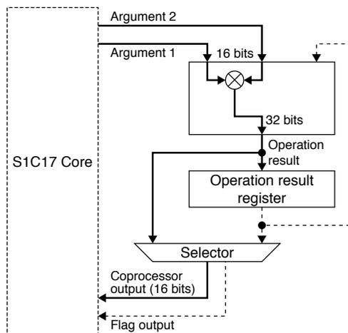
Figure 24.3.1 Data Path in Multiplication Mode
