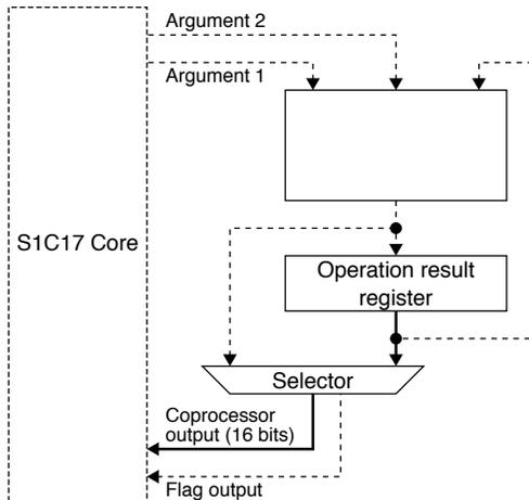
Figure 24.6.1 Data Path in Operation Result Read Mode
