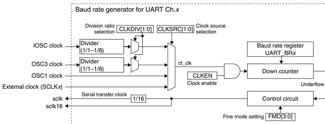
Figure 14.3.1 Baud Rate Generator
