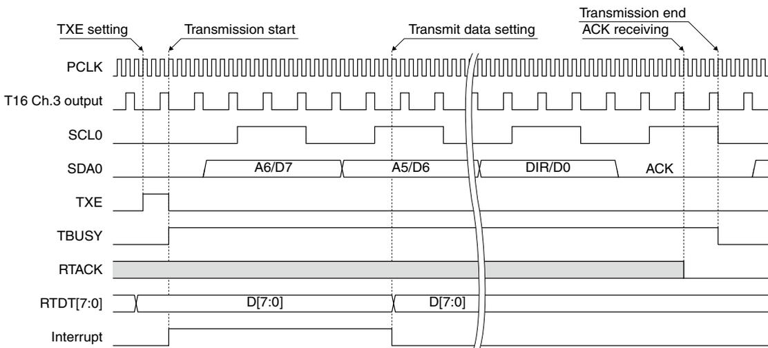
Figure 16.5.7 Slave Address Transmission/Data Transmission
