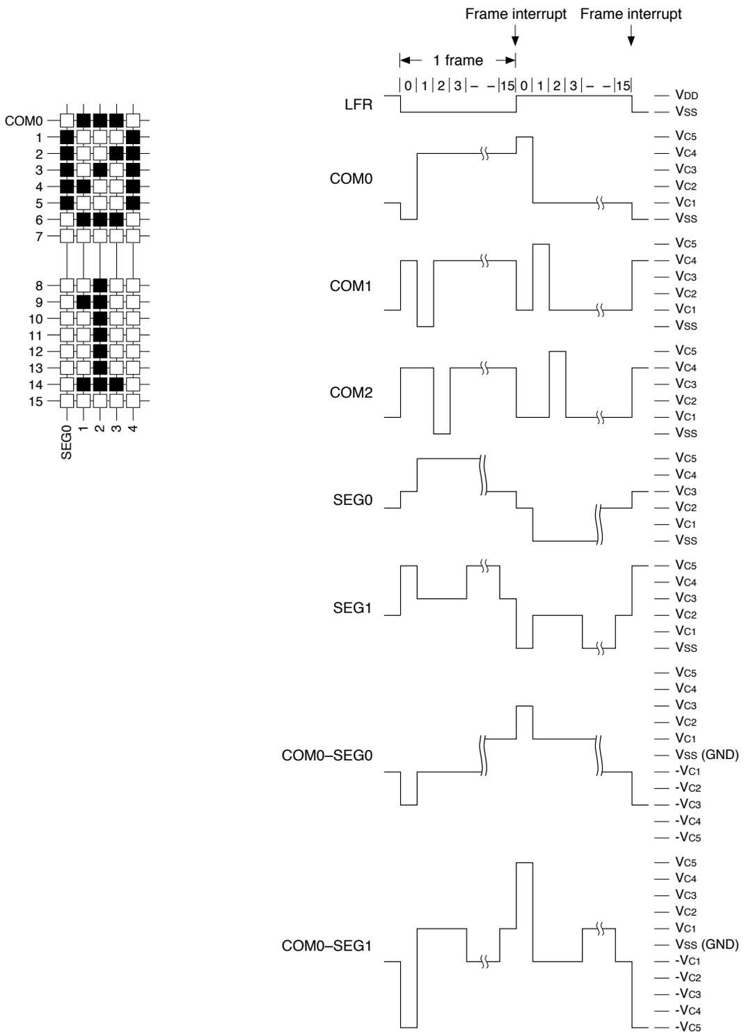
Figure 19.5.2.3 1/16 Duty Drive Waveform
