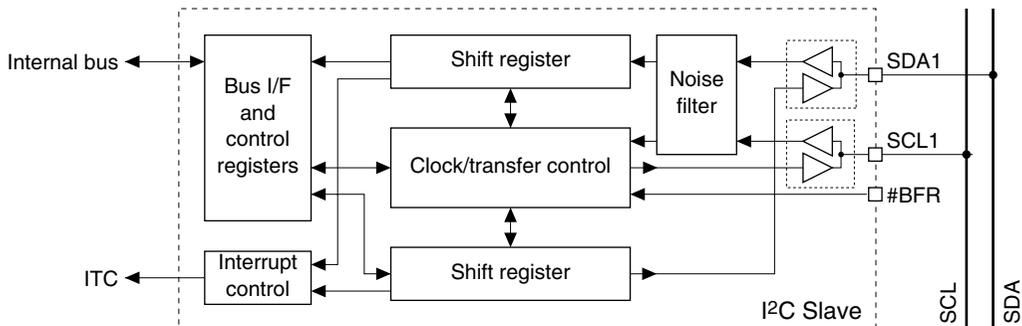
Figure 17.1.1 I2CS Module Configuration
