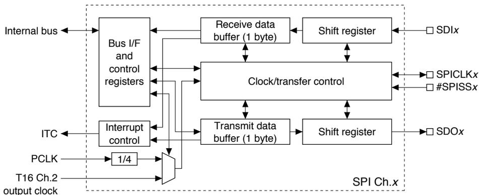
Figure 15.1.1 SPI Module Configuration (1 channel)
