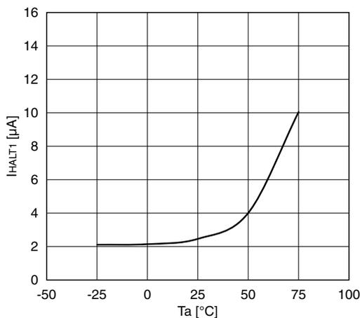
**Current consumption-temperature characteristic during execution with OSC1**
