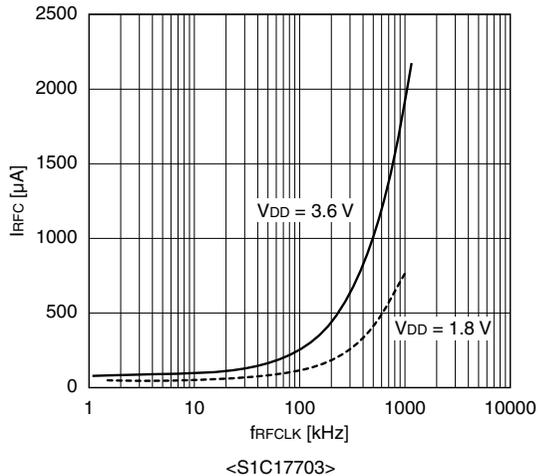
**RFC reference/sensor oscillation current consumption-frequency characteristic (Capacitive sensor DC oscillation mode)**
