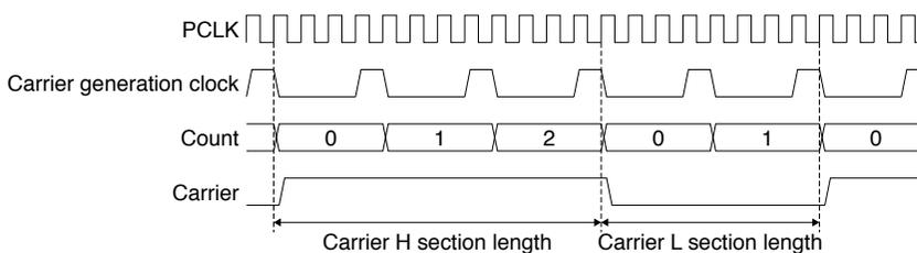
Figure 18.3.1 Carrier Signal Generation
