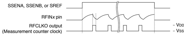
Figure 21.4.3.1 CR Oscillation Clock (RFCLK) Waveform
