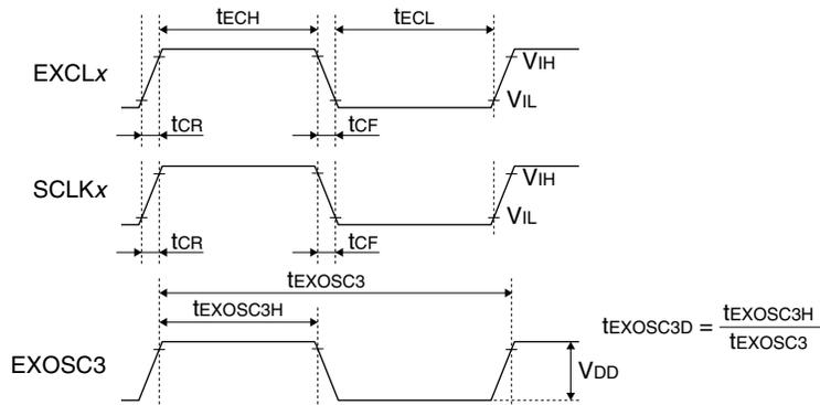
Figure 25.5.1 External Clock Input Timing
