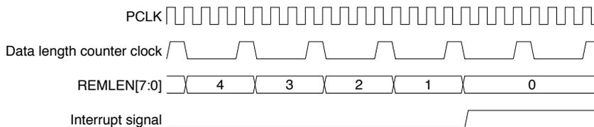
Figure 18.5.2 Underflow Interrupt Generation Timing
