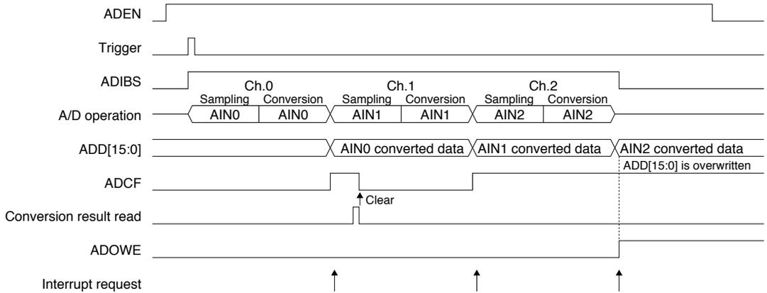
(2) Multi-channel (AIN0–AIN2) one-time conversion mode (ADCS = 0, ADCE = 2, ADMS = 0)
