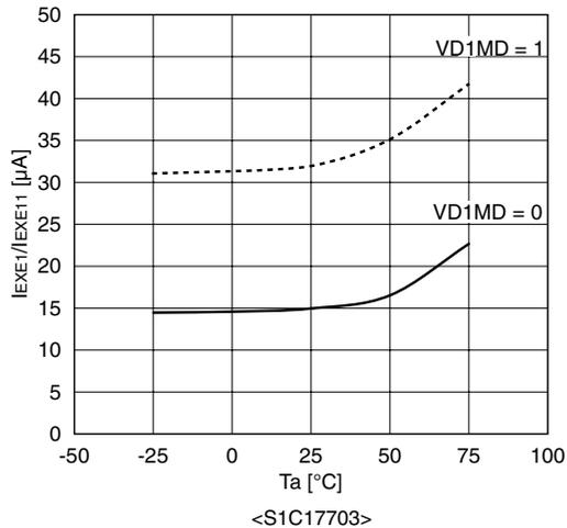
**Current consumption-temperature characteristic during execution with OSC1 + clock gear**
