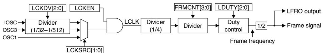
Figure 19.4.1 LCD Clock System
