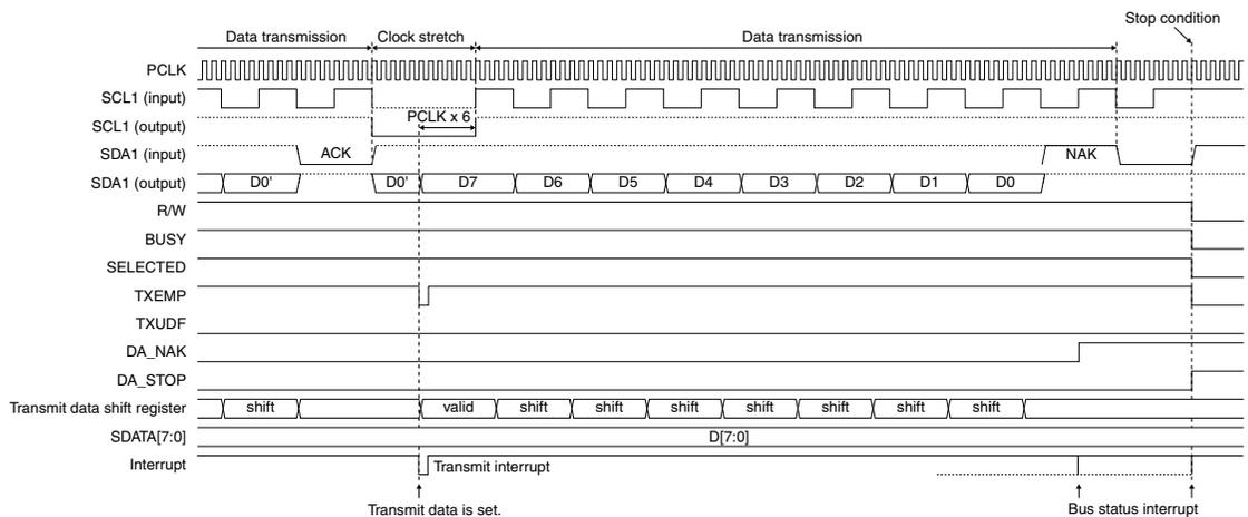
Figure 17.5.6 I<sup>2</sup>C Timing Chart 2 (data transmission → stop condition)
