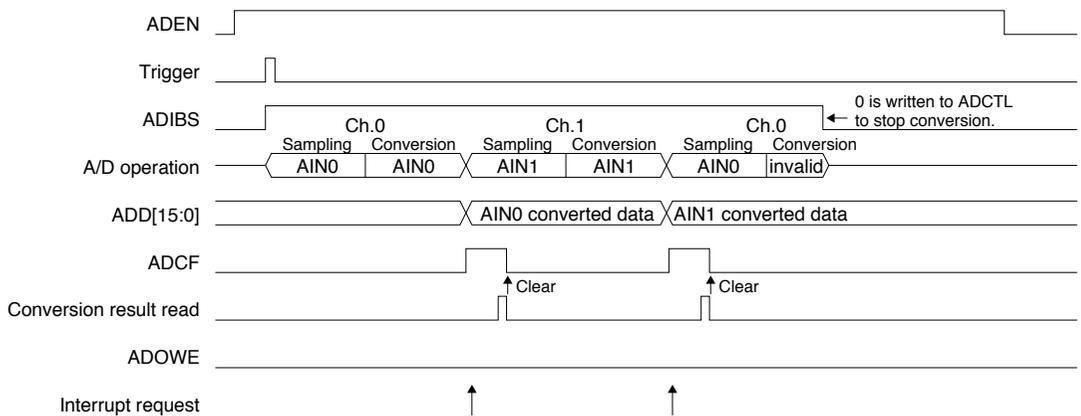
(4) Multi-channel (AIN0–AIN1) continuous conversion mode (ADCS = 0, ADCE = 1, ADMS = 1)
