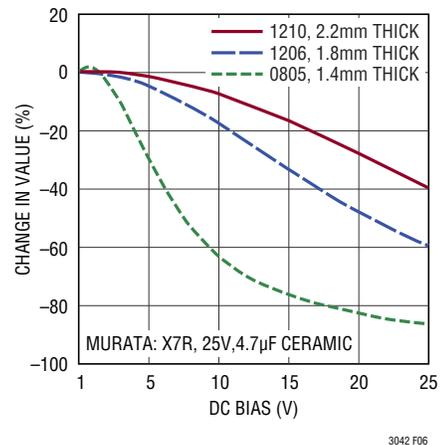
Figure 6. Capacitor Voltage Coefficient for Different Case Sizes
