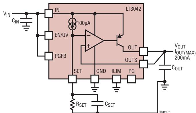
Figure 3.  $C_{OUT}$  and  $C_{SET}$  Connections for Stability
