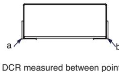
All soldering surfaces coplanar within 0.10 millimeters.
