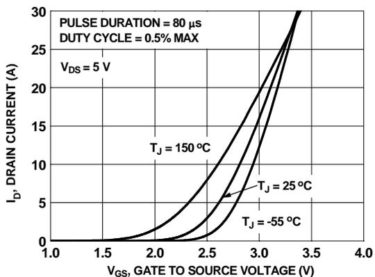
Figure 5. Transfer Characteristics
