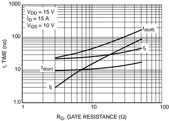
Figure 9. Resistive Switching Time Variation vs. Gate Resistance
