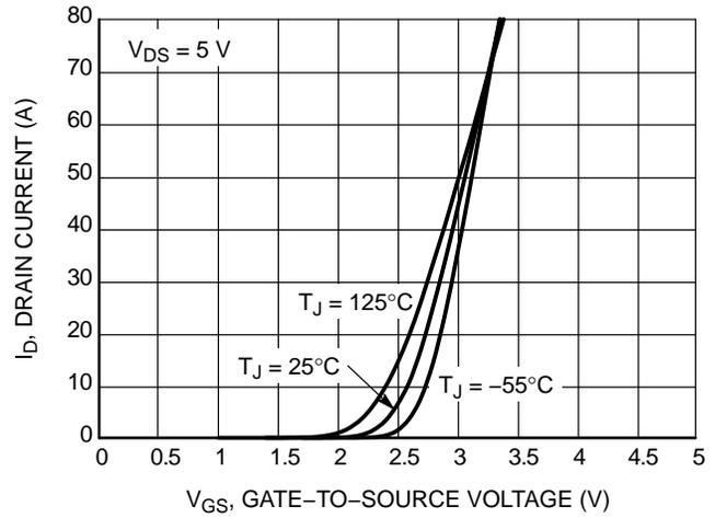
Figure 2. Transfer Characteristics
