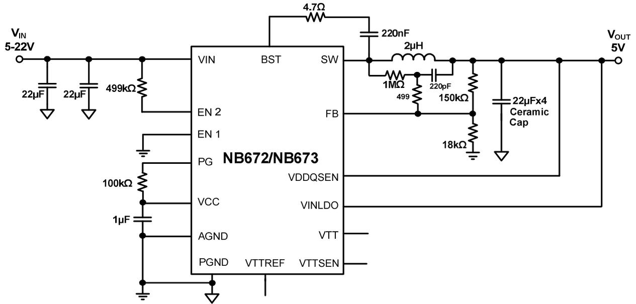
**Figure 16 – Typical Application Circuit with Low ESR Ceramic Output Capacitor**
