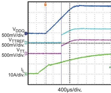
**V<sub>TT</sub> & V<sub>TTREF</sub> Shutdown through VIN**
