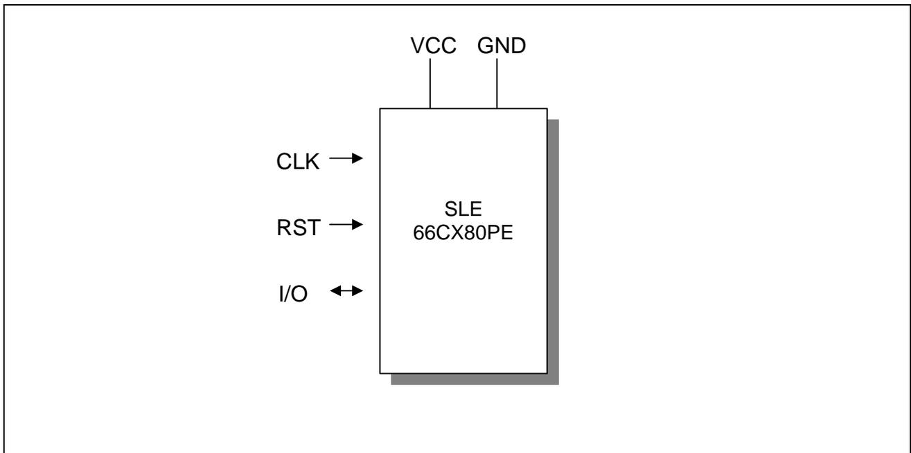
**Figure 1: Pin Configuration**
