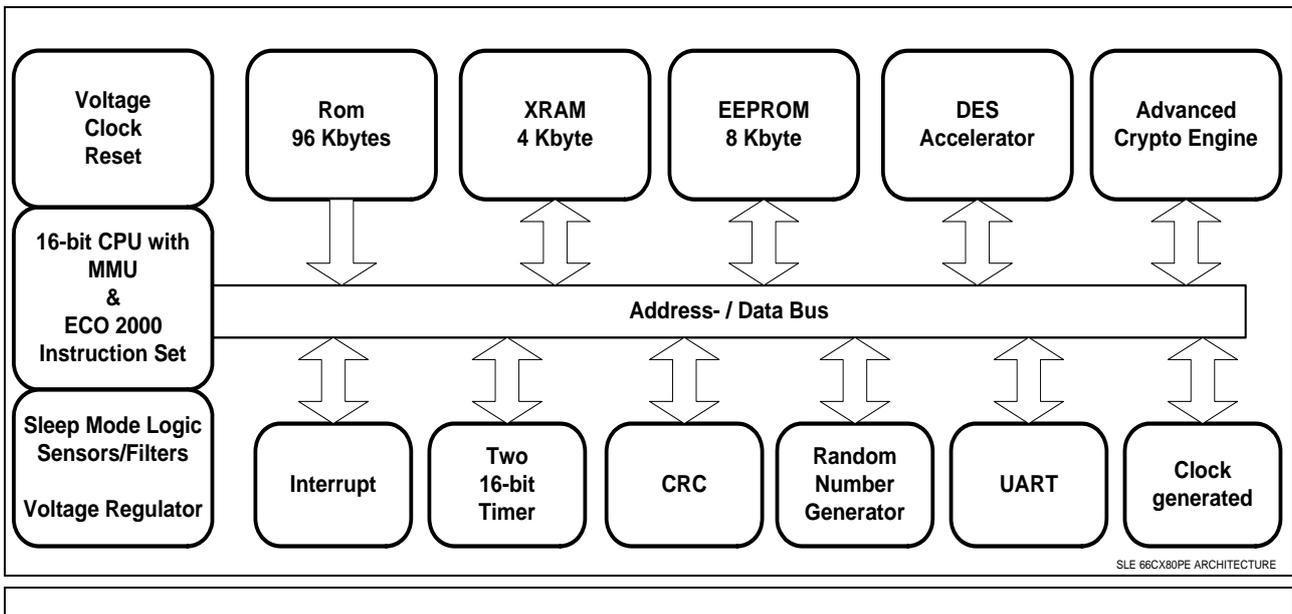
**Figure 2: Block Diagram SLE 66CX80PE**
