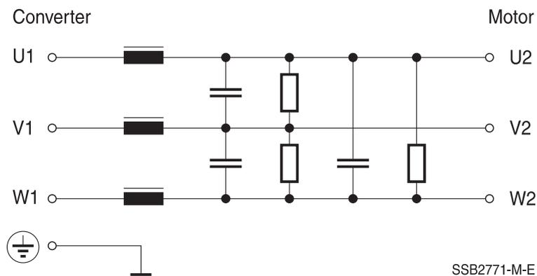
Sine-wave output filters for 3-phase systems
