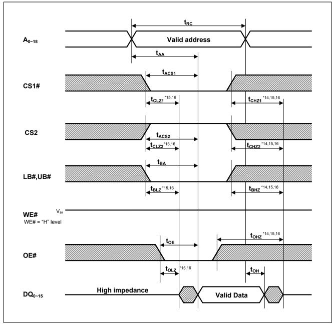
Note 14.  $t_{CHZ1}$ ,  $t_{CHZ2}$ ,  $t_{BHZ}$  and  $t_{OHZ}$  are defined as the time when the DQ pins enter a high-impedance state and are not referred to the DQ levels.
