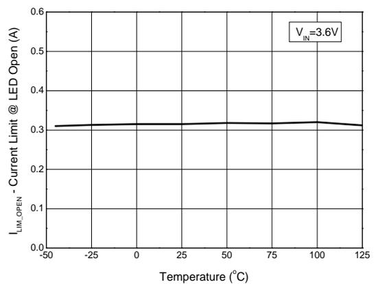
**Performance Characteristics** ( $V_{IN} = 3.6V$ ,  $L = 22\mu H$ ,  $R_{FB} = 10\Omega$ , 8 LEDs in series,  $T_A = +25^\circ C$ , unless otherwise specified.)
