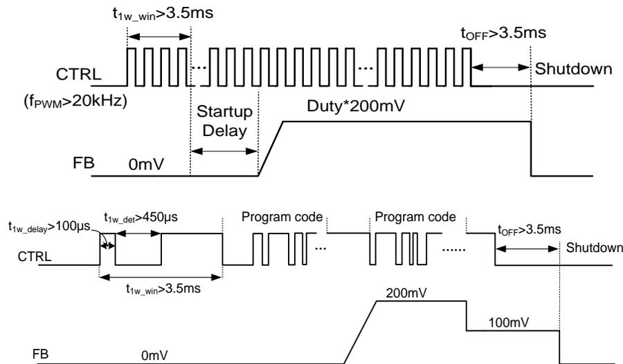
Figure 1. Dimming Mode Detection and Soft Start
