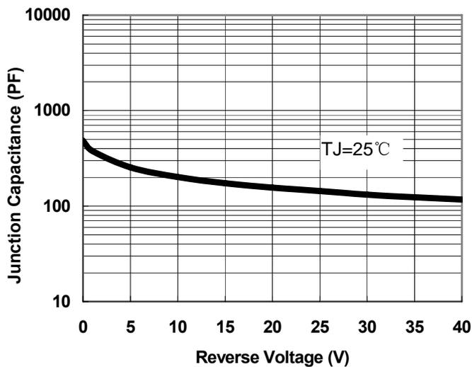
Fig.1-Typical Junction Capacitance
