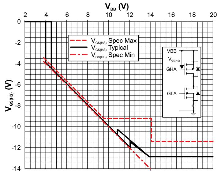
Figure 4: Typical High-Side Gate Drive vs. V<sub>BB</sub>
