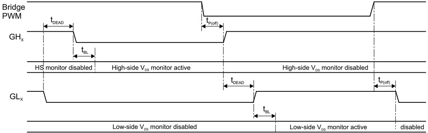
Figure 5: VDS Fault Monitor – Blank Mode Timing (VDQ = 1)
