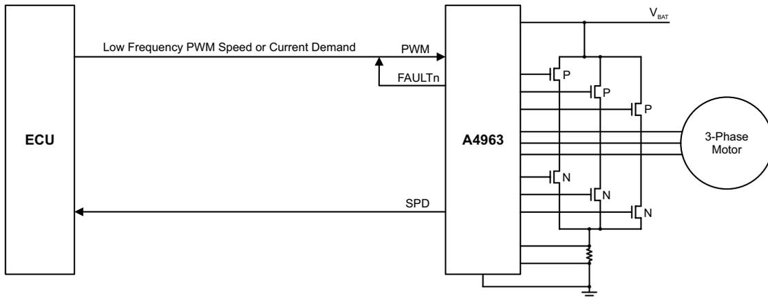
**Figure 10: Remote Single-Wire Command with Integrated Closed-Loop Control**
