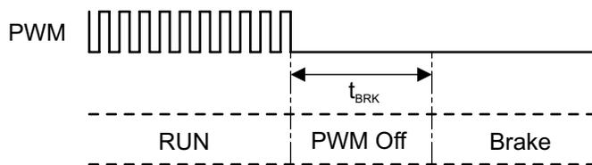
**Figure 12: PWM Brake Timing – Direct Mode PWM**
