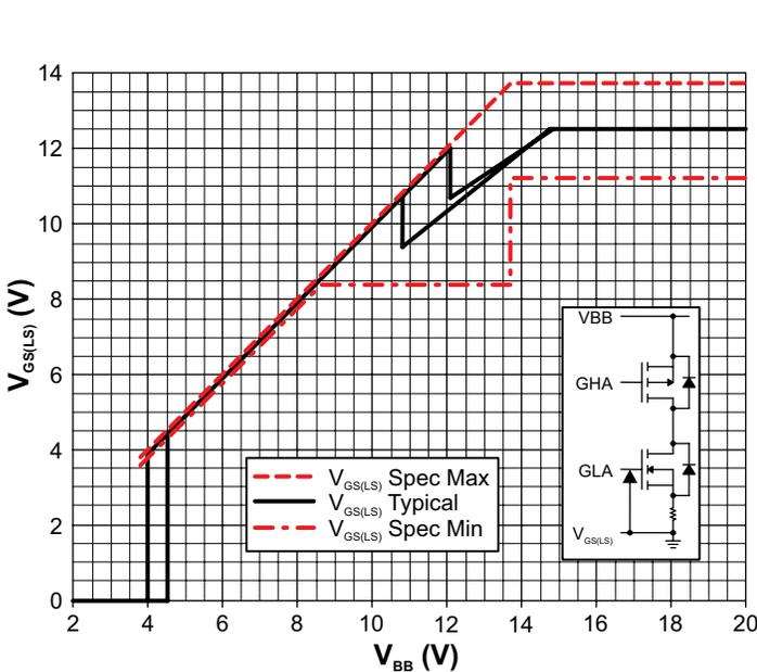
Figure 3: Typical Low-Side Gate Drive vs. V<sub>BB</sub>
