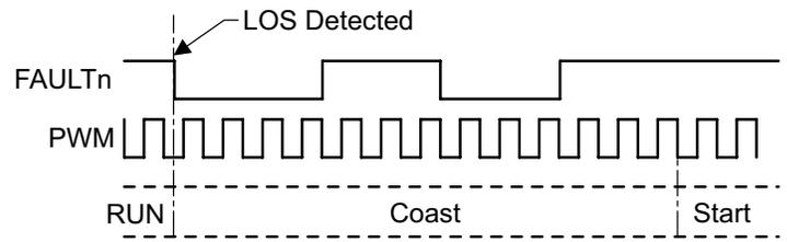
**Figure 14: LOS Fault Reporting - Indirect Mode PWM**
