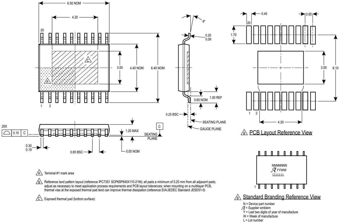
Figure 24: Package LP, 20-Pin TSSOP with Exposed Pad
