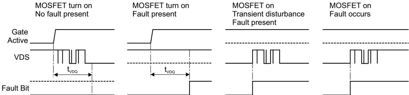
Figure 6: VDS Fault Monitor – Blank Mode Timing (VDQ = 1)
