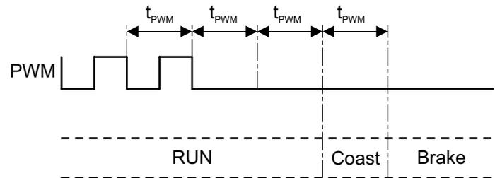
**Figure 15: PWM Brake Timing - Indirect Mode PWM**
