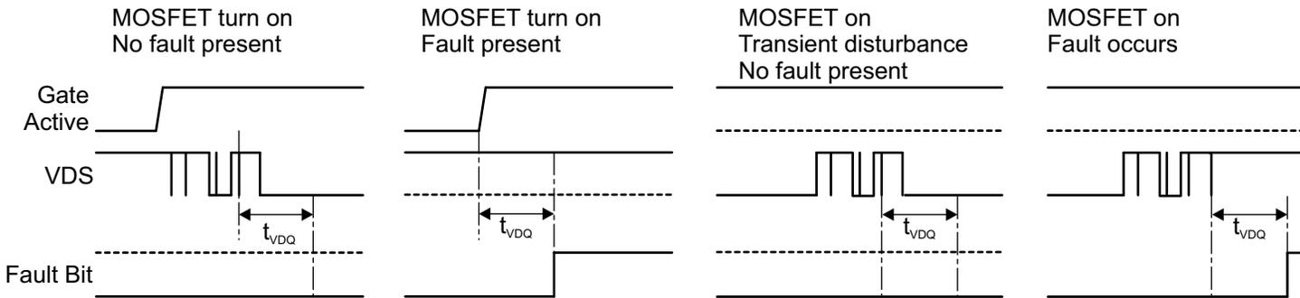
Figure 7: VDS Fault Monitor – Debounce Mode Timing (VDQ = 0)
