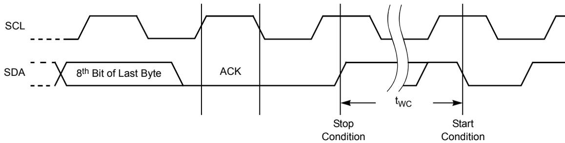
**Nonvolatile Write Cycle Timing**
