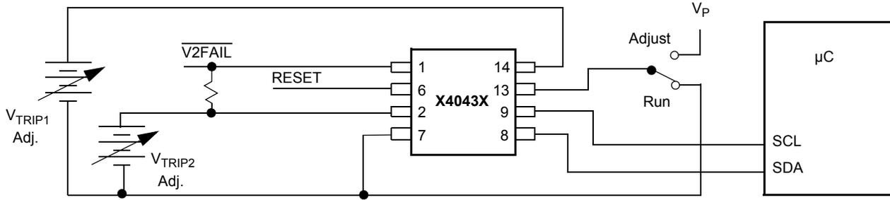
Figure 6. V<sub>TRIPX</sub> Set/Reset Sequence (X = 1, 2, 3)
