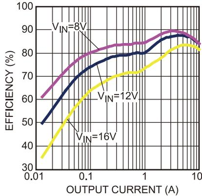
**Figure 16 — Efficiency Curve**
