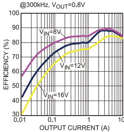
**Figure 22 — Efficiency Curve**
