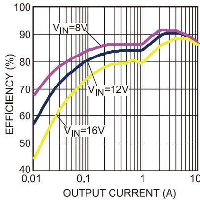
Figure 32 — Efficiency Curve
