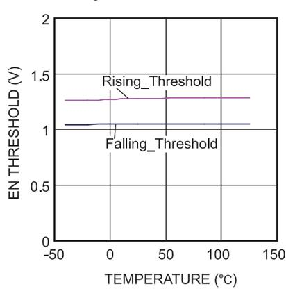
**V<sub>CC</sub> UVLO Threshold vs. Temperature**
