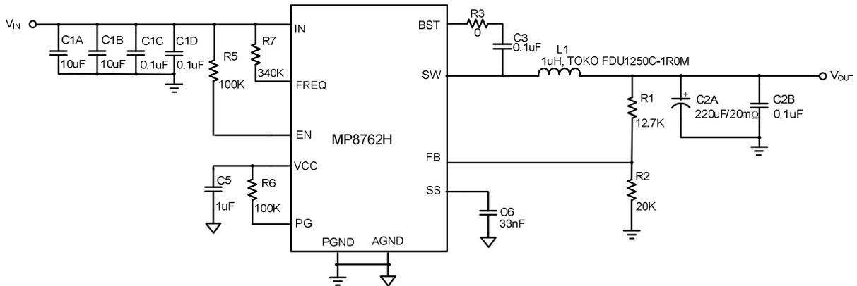
**Figure 13 — Typical Application Circuit with No External Ramp**
