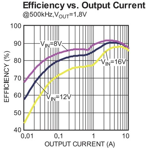
**Figure 40 — Efficiency Curve**
