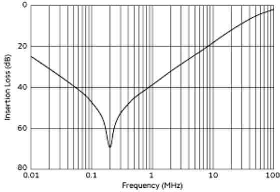
Common Mode Insertion Loss (Typ.)
