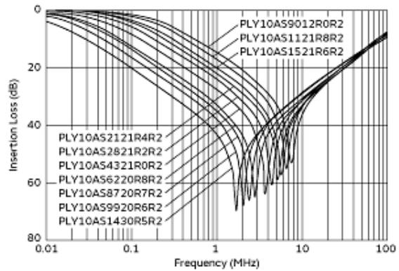
Differential Mode Insertion Loss-Frequency Characteristics
