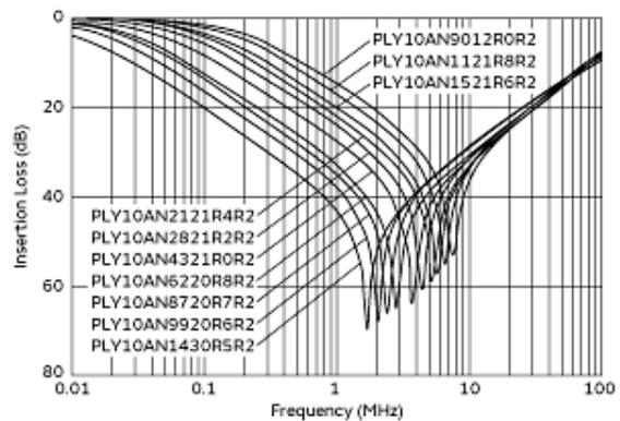
Differential Mode Insertion Loss-Frequency Characteristics
