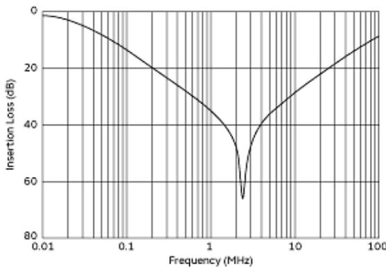
Differential Mode Insertion Loss (Typ.)
