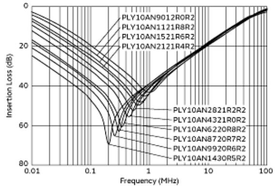
Common Mode Insertion Loss-Frequency Characteristics
