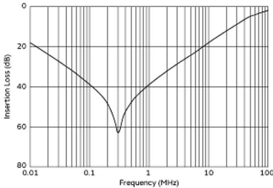
Common Mode Insertion Loss (Typ.)
