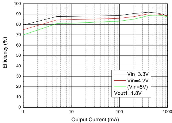
OUT2 Efficiency vs. Output Current
