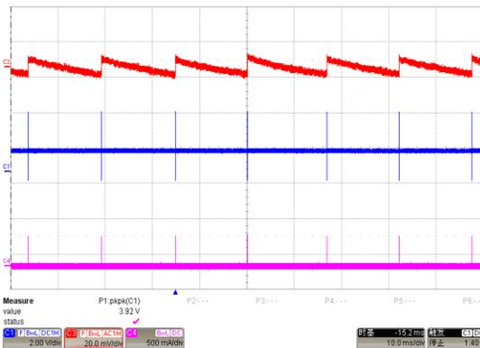
(CH1=Switch; CH3=Output Voltage; CH4=Inductor current)
