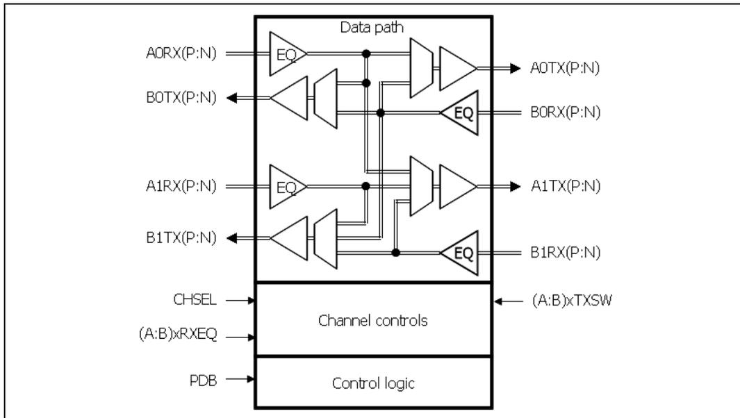
Figure 2 Block Diagram
