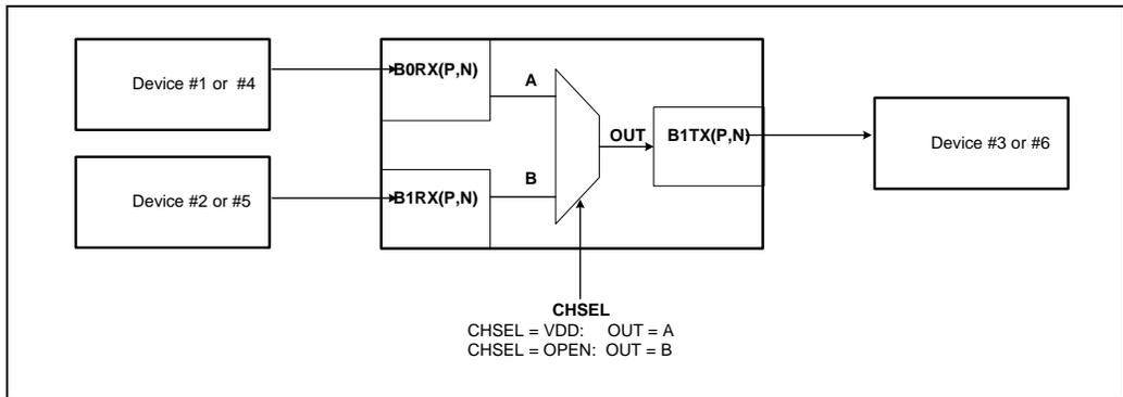
Figure 7 Implementation of Second Instance of Unidirectional 2:1 Mux
