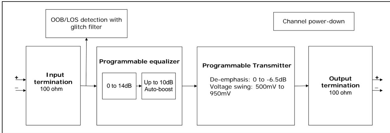
Figure 3 Channel Block Diagram with Channel Features
