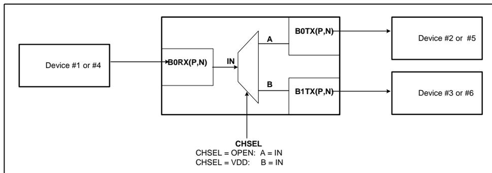
Figure 9 Implementation of Second Instance of Unidirectional 1:2 De-Mux
