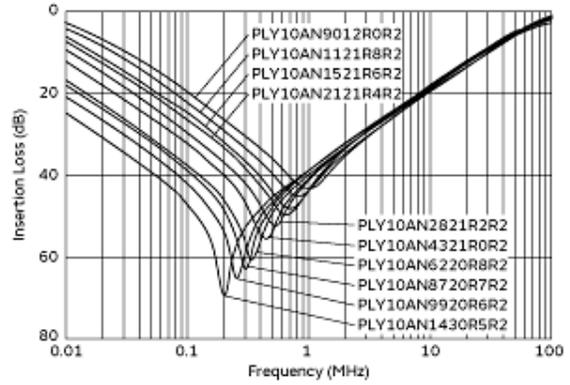
Common Mode Insertion Loss-Frequency Characteristics
