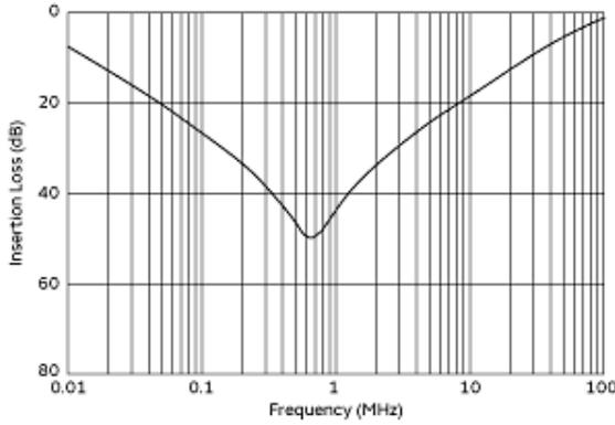
Common Mode Insertion Loss (Typ.)
