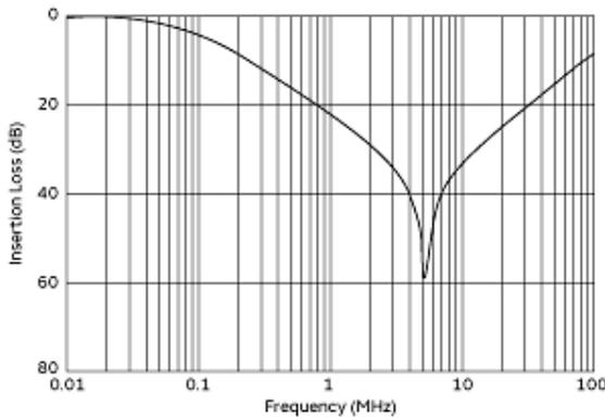
Differential Mode Insertion Loss (Typ.)
