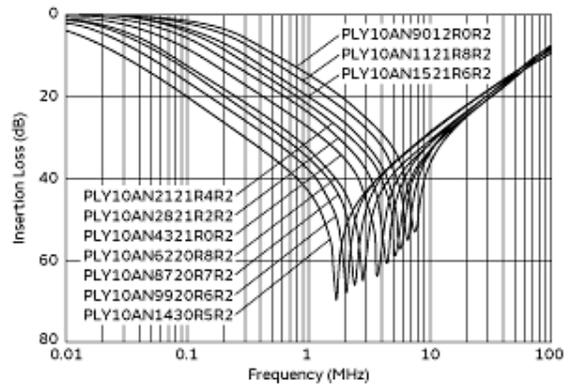
Differential Mode Insertion Loss-Frequency Characteristics
