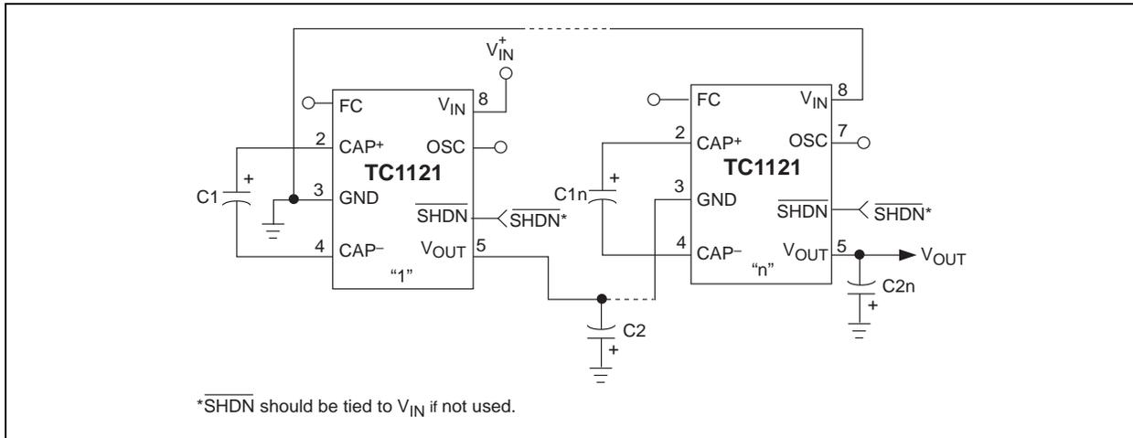
**FIGURE 3-2:** Cascading TC1121s to Increase Output Voltage
