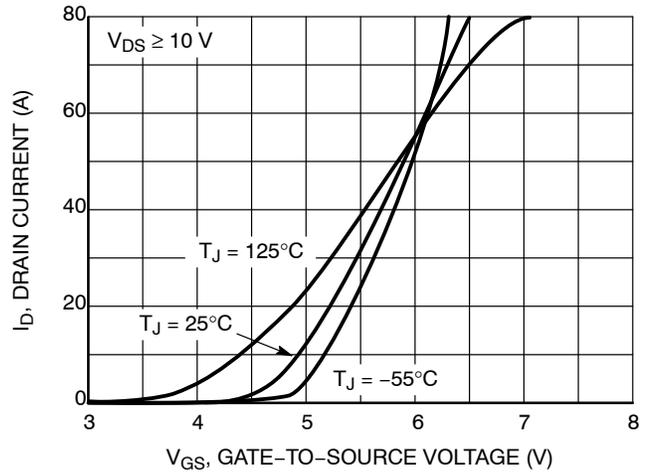
Figure 2. Transfer Characteristics
