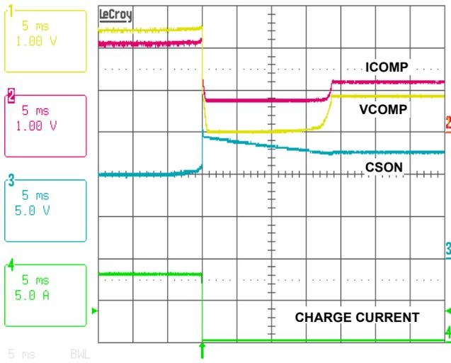
FIGURE 17. BATTERY REMOVAL
