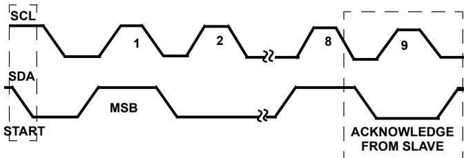
FIGURE 24. ACKNOWLEDGE ON THE I<sup>2</sup>C BUS
