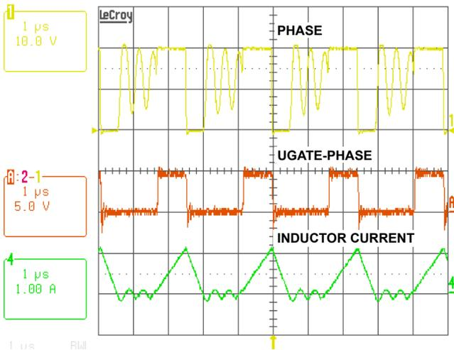
**FIGURE 13. SWITCHING WAVEFORMS IN DIODE EMULATION MODE**
