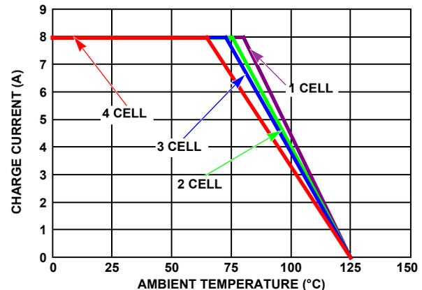
FIGURE 2. DERATING CURVE WITH NATURAL AIR FLOW (MEASURED ON 10cm x 10cm EVALUATION BOARD)
