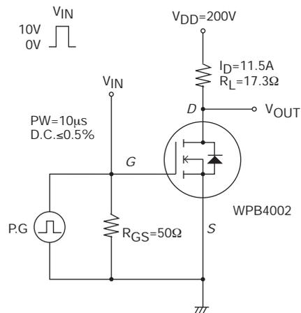
Fig.3 trr Reverse Recovery Resistance Test Circuit
