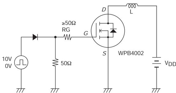
Fig.2 Switching Time Test Circuit
