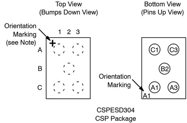
Note: Lead-free devices are specified by using a "+" character for the top side orientation mark.
