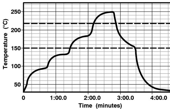
Figure 4. Lead-free (SnAgCu) Solder Ball Reflow Profile
