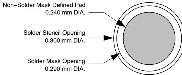
Figure 3. Recommended Non-Solder Mask Defined Pad Illustration
