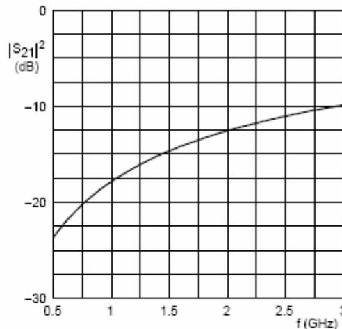
Diode zero biased and inserted in series with a  $50 \text{ } \Omega$  stripline circuit.
