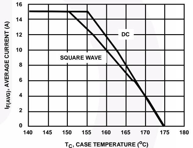
FIGURE 4. 6. TYPICAL CURRENT DERATING CURVE vs CASE TEMPERATURE
