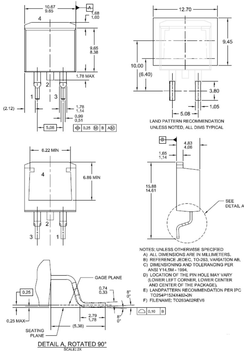
**Figure 9. TO-263 2L (D<sup>2</sup>-PAK) - 2LD, TO263, SURFACE MOUNT**
