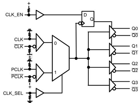
Figure 1. Simplified Logic Diagram of NB3L8533
