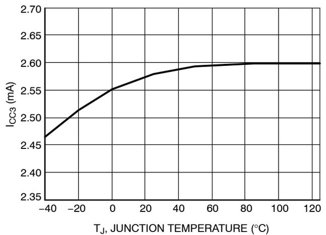
Figure 8. I<sub>CC3</sub> vs. Junction Temperature
