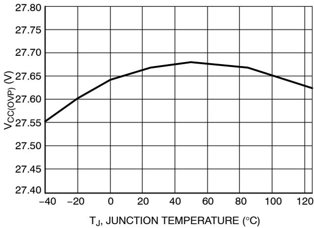
Figure 5. V<sub>CC(OVP)</sub> vs. Junction Temperature
