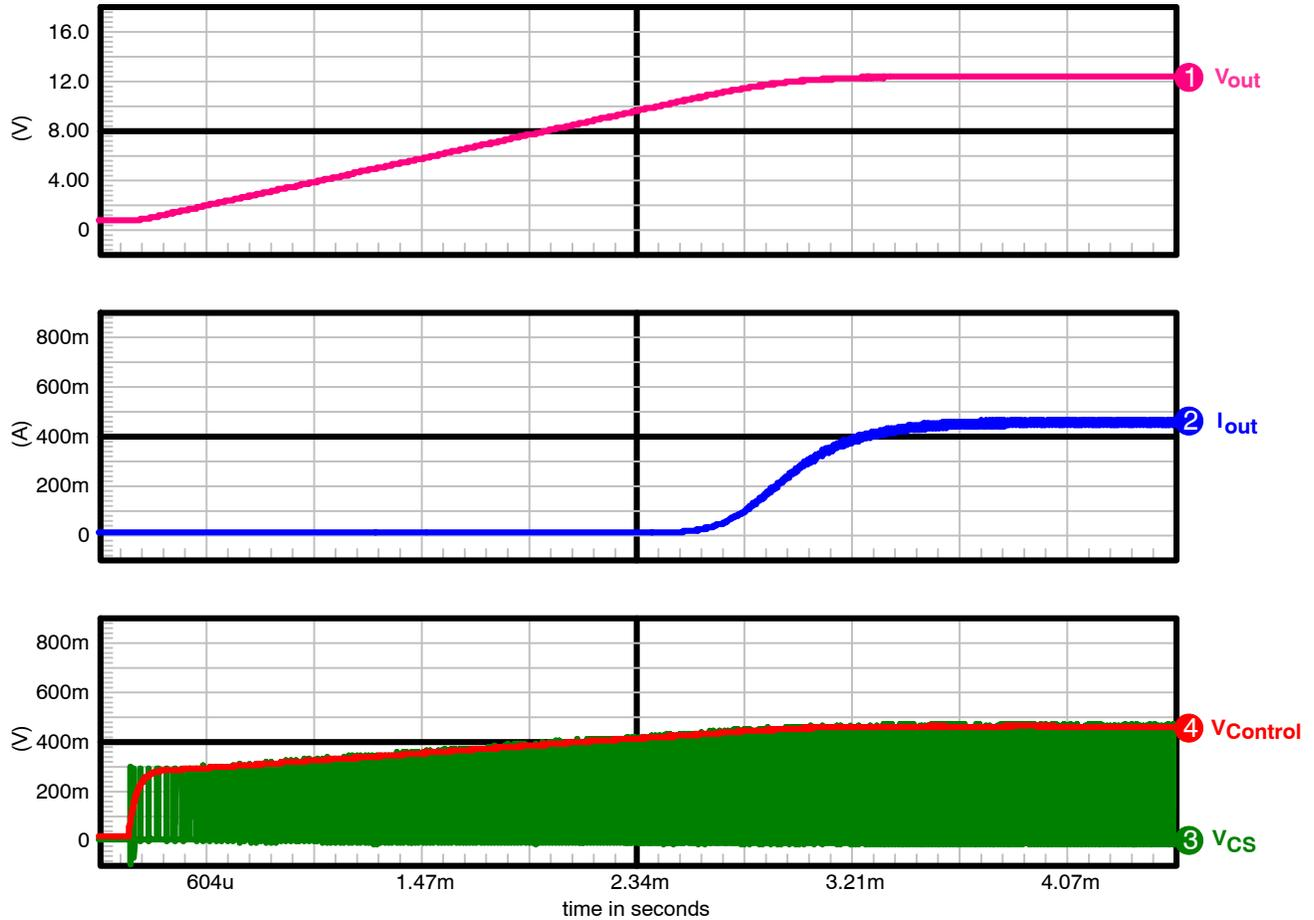
**Figure 29. Startup Simulation Showing the Natural Soft-start**
