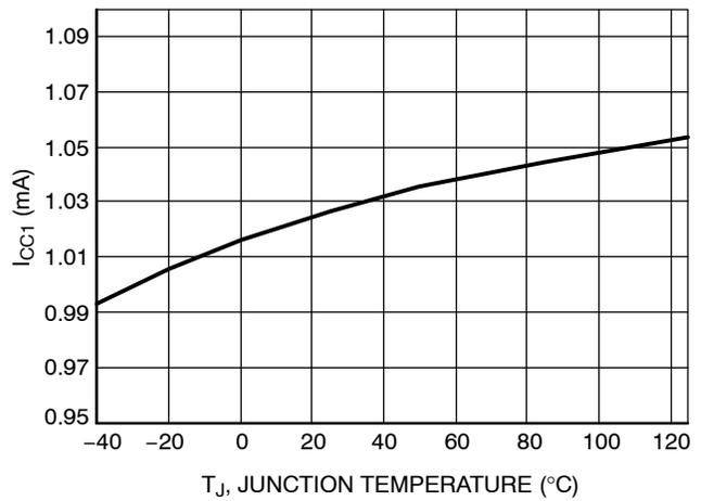
Figure 6. I<sub>CC1</sub> vs. Junction Temperature
