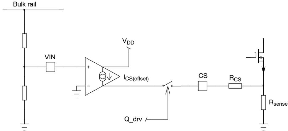
**Figure 34. Line Feed-forward Schematic**
