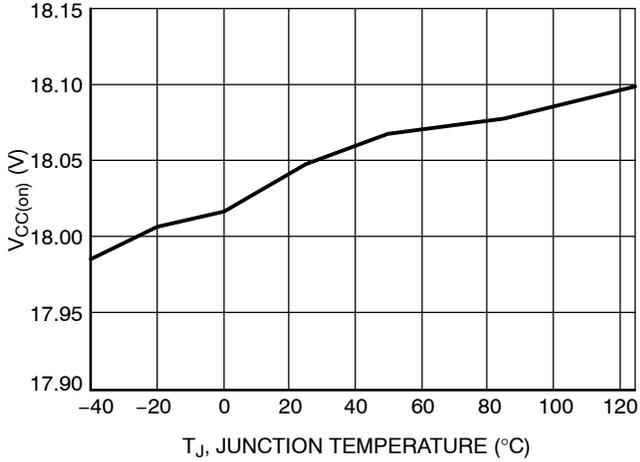
Figure 3. V<sub>CC(on)</sub> vs. Junction Temperature
