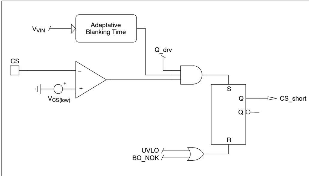
**Figure 37. CS Pin Short Circuit Protection Schematic**
