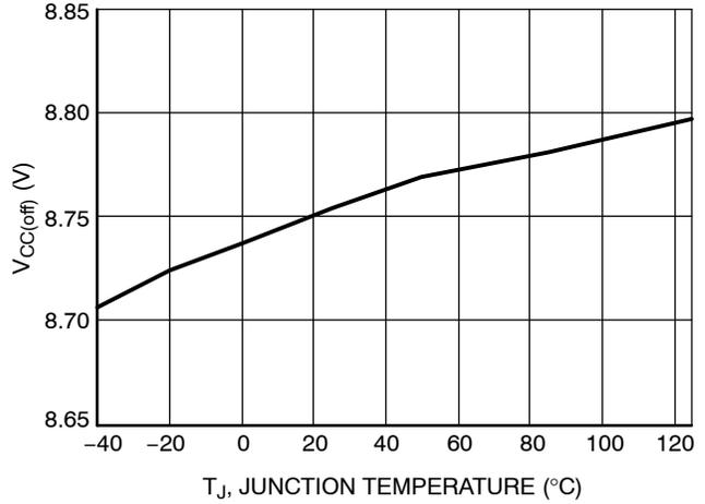
Figure 4. V<sub>CC(off)</sub> vs. Junction Temperature
