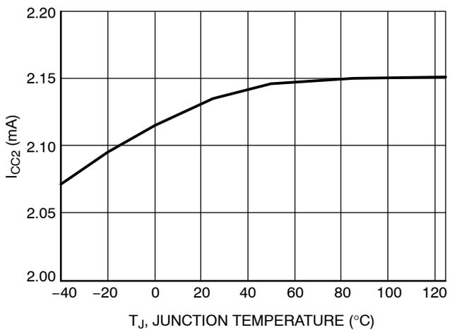
Figure 7. I<sub>CC2</sub> vs. Junction Temperature
