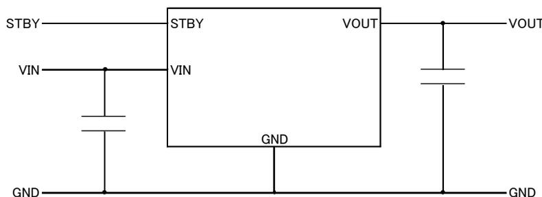
Fig.1 Application Circuit
