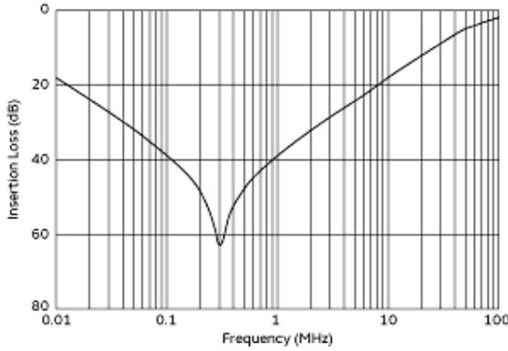
Common Mode Insertion Loss (Typ.)
