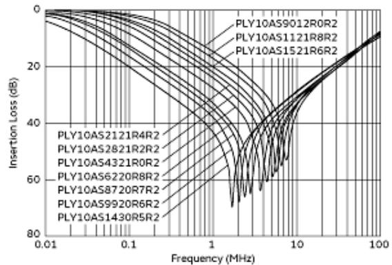
Differential Mode Insertion Loss-Frequency Characteristics
