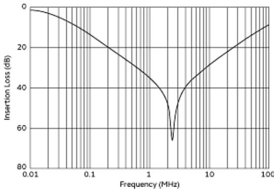
Differential Mode Insertion Loss (Typ.)
