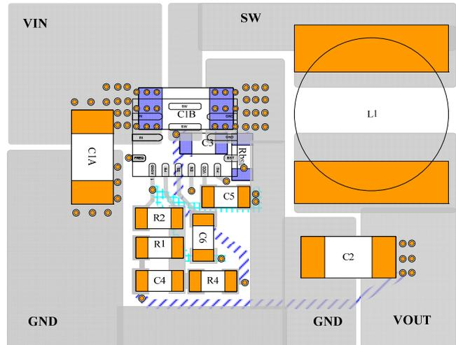
**Figure 16—PCB LAYOUT**
