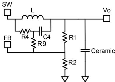
**Figure8—Simplified Circuit of Ceramic Capacitor**
