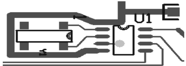
FIGURE 12. SUGGESTED LAYOUT FOR ISL12057 AND CRYSTAL
