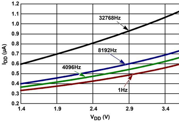
FIGURE 4. I<sub>DD</sub> vs V<sub>DD</sub> vs F<sub>OUT</sub>
