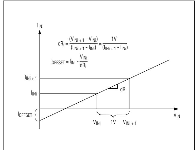
Figure 2. Effective Differential Resistance and Offset Current
