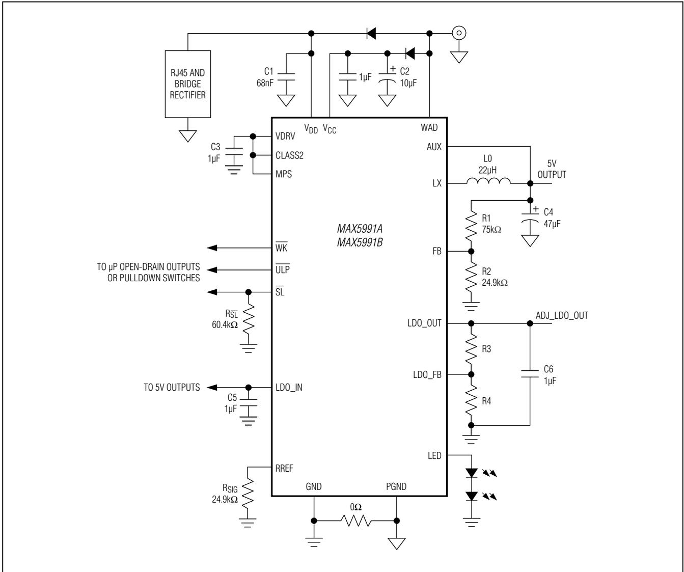
Figure 4. MAX5991A/MAX5991B 5V Buck Regulator and Adjustable LDO
