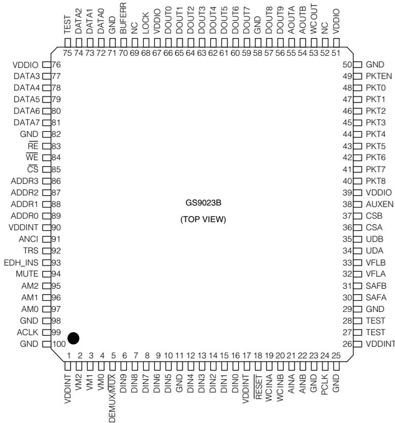
NOTE: The GS9023B DOUT[9:0] MSB to LSB convention is compatible with the GS9022 but reversed with the GS9032 or GS7005. See Interconnection with GS9032 or GS7005 section.
