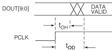
Figure 2-2: Video Data Output Delay & Hold Times
