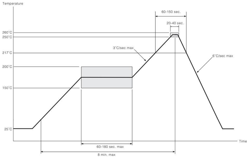
Figure 2-5: Maximum Pb-Free Solder Reflow Profile (Preferred)
