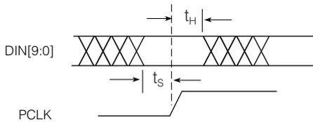
Figure 2-1: Video Data Input Setup & Hold Times
